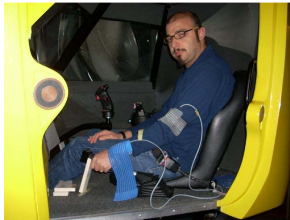
Figure 11: Experimental test set-up with acceleration sensors applied to the arm of the pilot
