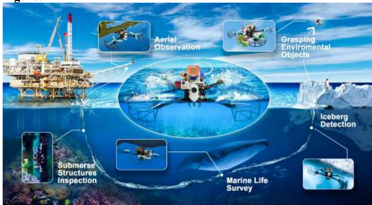
Fig. 1. A depiction of the mission profile and design of an aerial-aquatic hitchhiking robot. The robot's ability to transition across water and air and attach robustly to a wide variety of surfaces allows it to perform long-term missions (such as monitoring) in natural environments. All image elements from the third party are approved with licenses.
