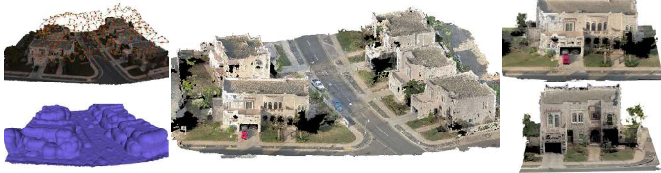
Fig. 1. Proposed method and results of aerial path planning. We first compute an optimal aerial flight trajectory from an initially reconstructed nadir capture. A safe airspace (everything outside the purple region) in the lower left subfigure is created to allow the flight trajectory to descend much closer without collision. In the middle column we show the dense reconstruction of one of the field tests and on the right close ups of two of the reconstructed townhouses.
