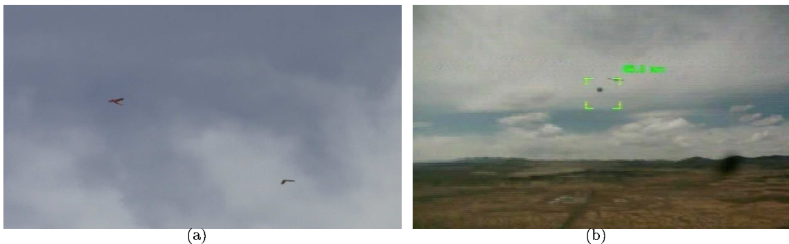
Fig. 11 (a) External video frame showing mothership and UAS in formation flight; (b) Single frame from UAS camera while following drogue. Drogue is visible in center of green acquisition box. Mothership is obscured by top right corner of acquisition box.
