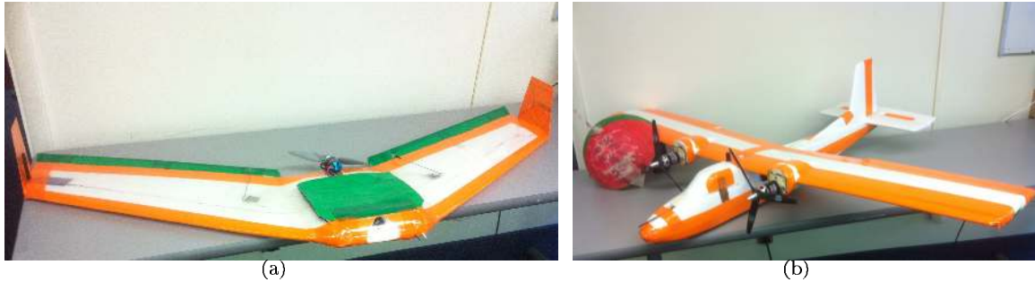
Fig. 9 (a) The model aircraft used as the seeker is a 1.4 m wingspan flying wing equipped with an autopilot, camera, and on-board vision processing unit. (b) Mothership and drogue. The drogue is a 30 cm diameter half-sphere towed using a nylon cable.
