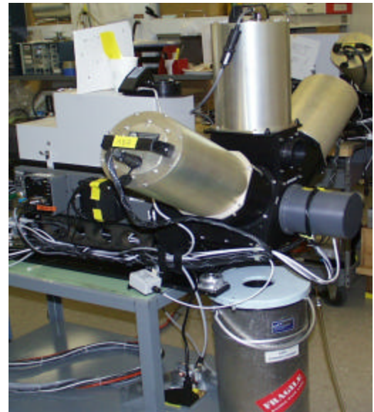
Figure 3. Laboratory tests of the calibration performance of an AERI instrument.
