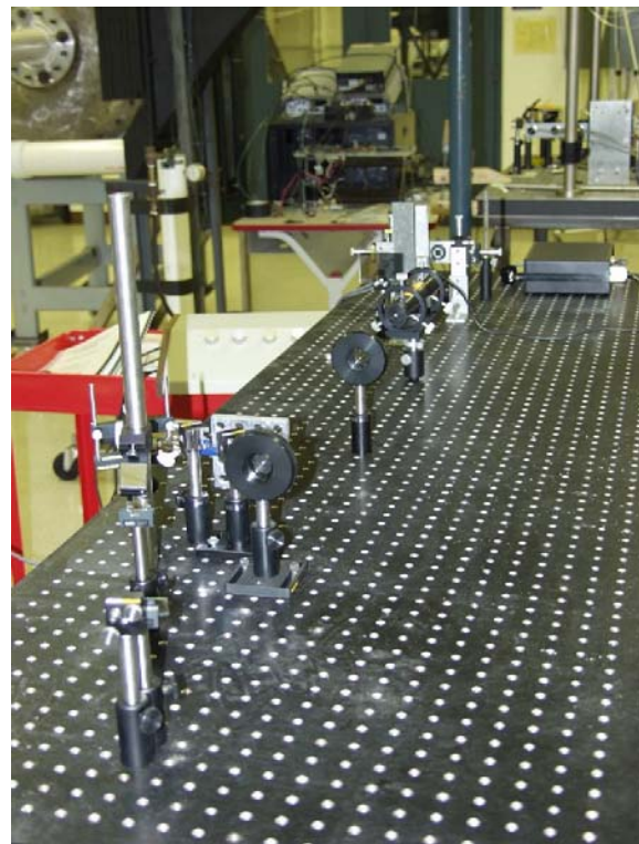
Figure 3. A Malley probe: schematic and actual set-up.
