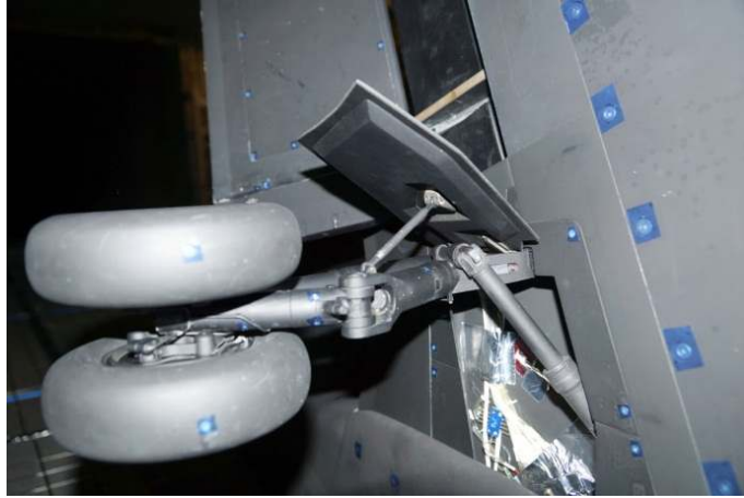
Figure 8. Frontal view of the baseline main landing (Goodrich) gear on 18% scale aircraft model.
