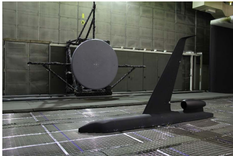
Figure 11. 14 x 22 tunnel test section showing array mounted in flyover position.
