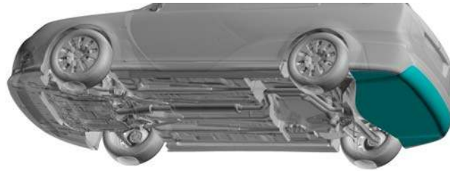
Figure 24: Configuration with only diffuser and underbody panel
