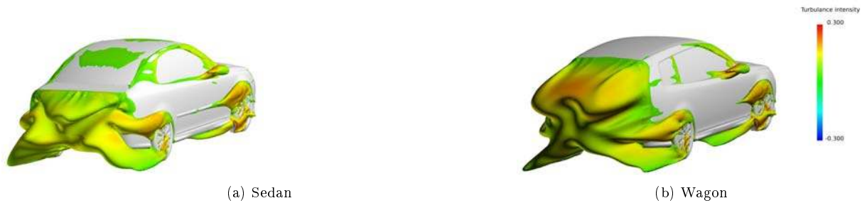
Figure 26: Iso-surface for total pressure equal to zero, here coloured with turbulence intensity
