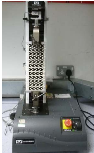
Figure 5. Tensile test of the rapid prototyped honeycomb core
