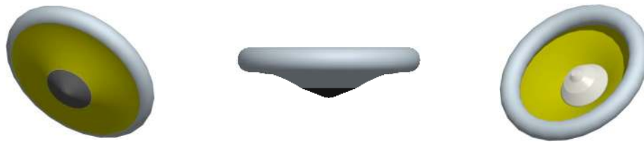
Figure 1. Tension cone inflatable aerodynamic decelerator.
