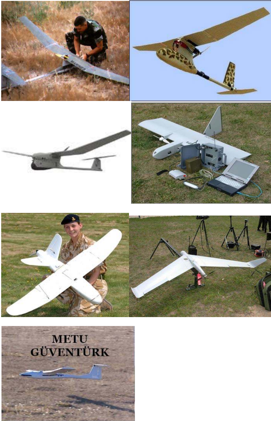
Fig. 22 Comparative UAVs: Photos of comparative small UAVs: these photos can help to have a visual understanding of the class of aircraft under consideration. From the top left to the bottom the pictures represent: Pointer, Raven, Puma, Dragon Eye, Desert Hawk, Orbiter and Metu Guventurk. From this pictures it can be also noticed the different layouts used for the different small UAV.
