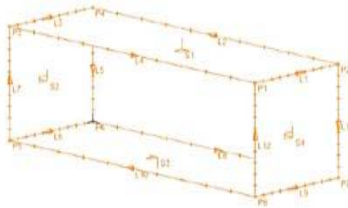
Fig.51 Adina: definition of the model: Using the finite element software ADINA, the first step is the definition of the model geometry. The points, the lines and the surfaces are defined, following the physical and geometric characteristics of the model. The model shown in this figure is model #1 with 0 stagger and 1 gap.
