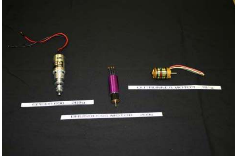
Fig. 27 Types of electric motors: There are 3 basic types of electric motors suitable for Small UAV applications and they are shown in this picture. On the left there is a traditional brushed motor. In the middle there is an inner brushless motor and on the right there is an outrunner brushless motor.
