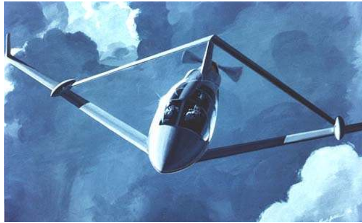
Fig 12 Joined wing configuration: This figure represents a Joined wing configuration. The shape of a joined wing configuration is obtained by attaching the forward wing low on the fuselage, then sweeping backward and upward while tapering it to the tip. The aft wing is attached high on the vertical fin.
