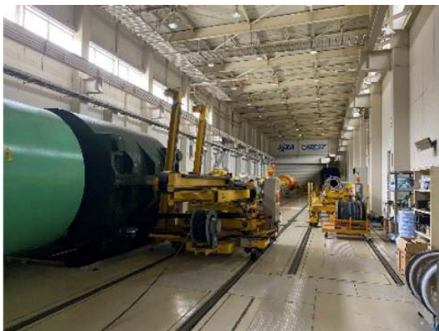
Fig. 6 Free-piston shock tunnel HIEST
