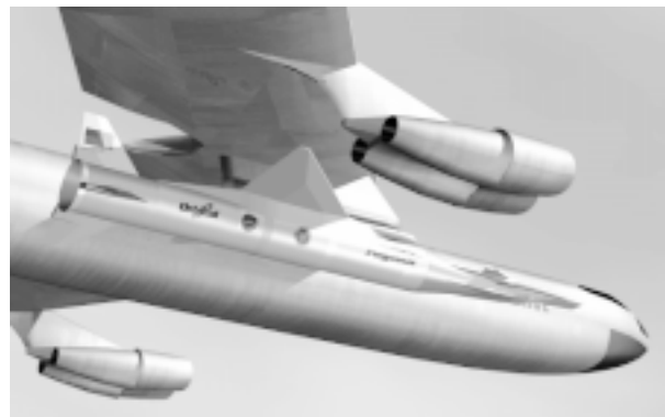
Figure 3. Artist's rendition of the HXLV being carried aloft on NASA's B-52 aircraft (from the Hyper-X flight profile video animation: http://lava.larc.nasa.gov/MOVIES/MEDIUM/LV-1997-00005.mov ).
