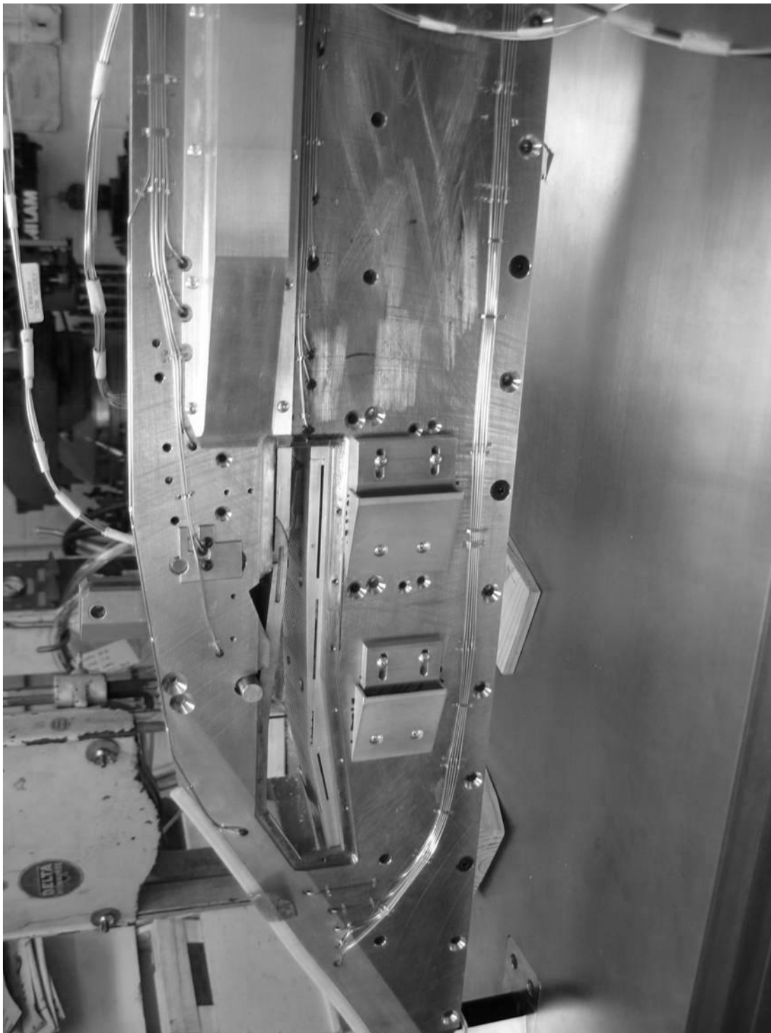
Figure 55. - Picture of low-speed inlet with sidewall bleed plate removed.
