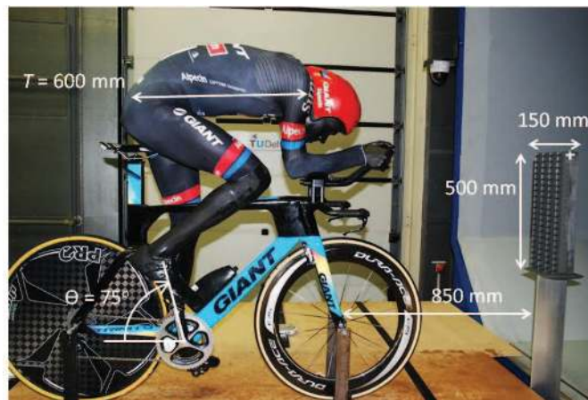
Fig. 2 Wind tunnel model and PIV seeding system.
