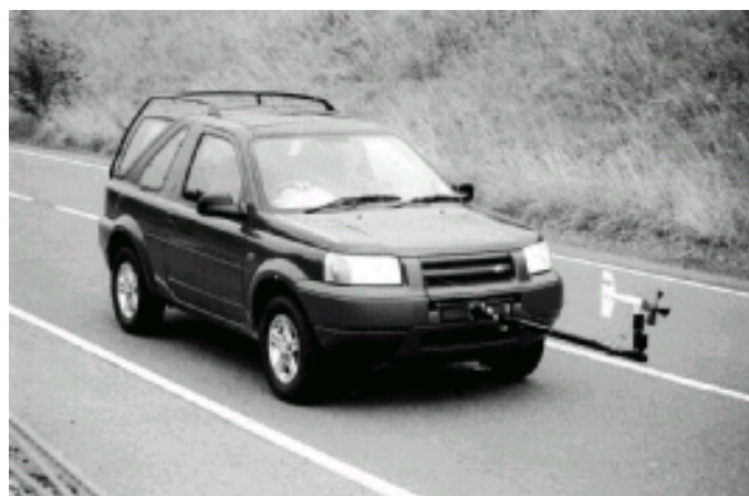
Figure 1. Land Rover Freelander during coastdown testing.
