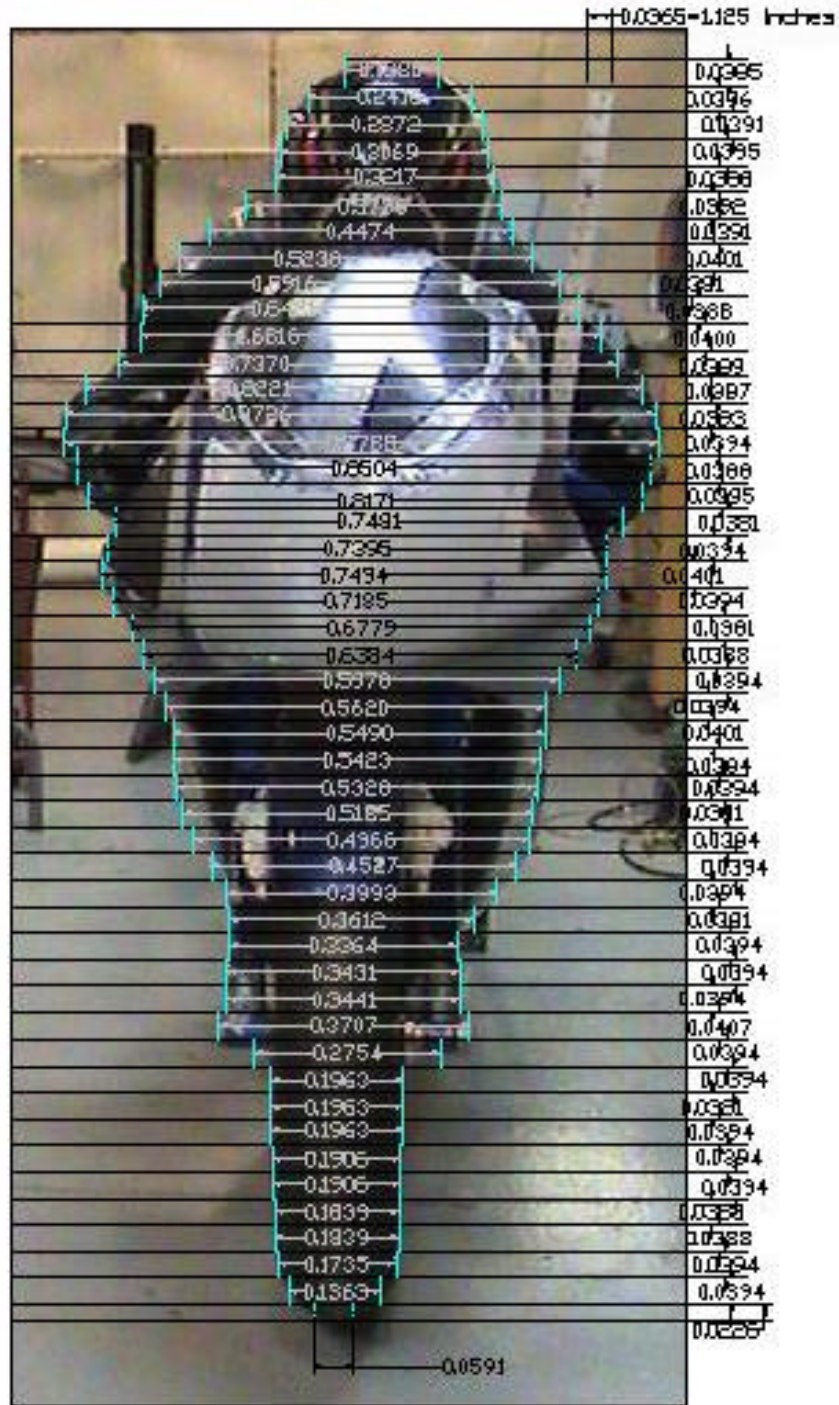
Figure 3.10: Frontal View of Tul-Aris Model for Frontal Area Determination.
