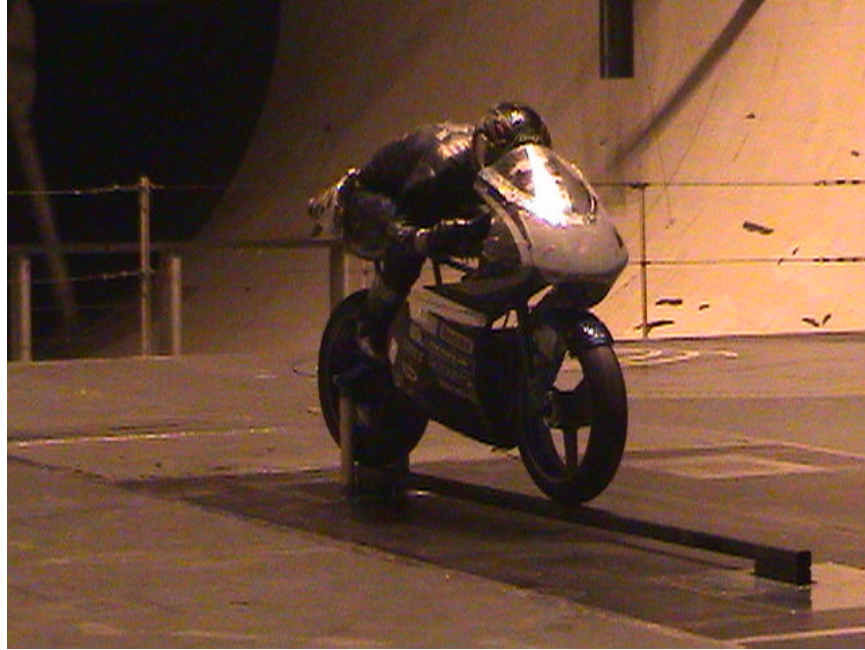
Figure 3.15: Photograph of the Tul-Aris Model and Sting Installed in the Langley Full Scale Tunnel.
