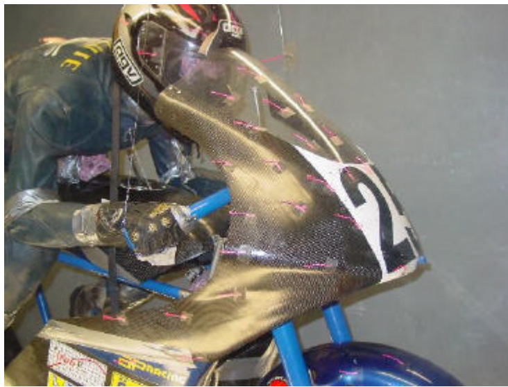
Figure 4.1: Initial Shape of the Upper Fairing of the Tul-Aris Motorcycle.
