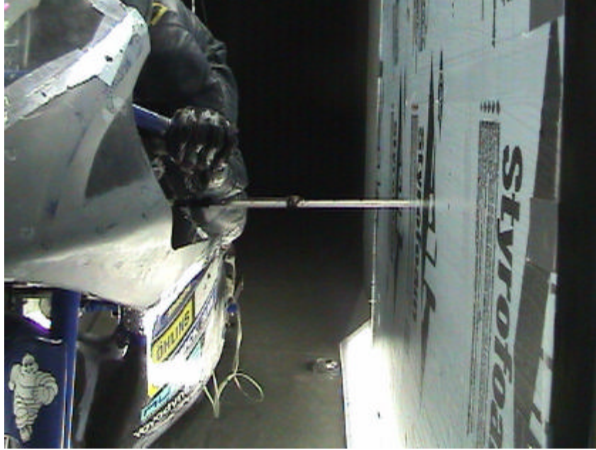
Figure 3.14: Photograph of Pitot-Static Tube installed along the Side of the Model near the Location of Maximum Thickness During the Increased Blockage Test.
