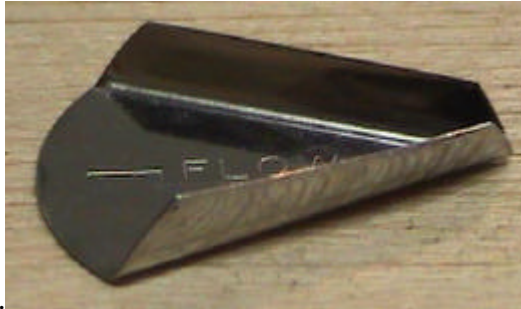
Figure 3.5: Modified 1/4-inch Vortex Generator. A. Front View B. Side View
