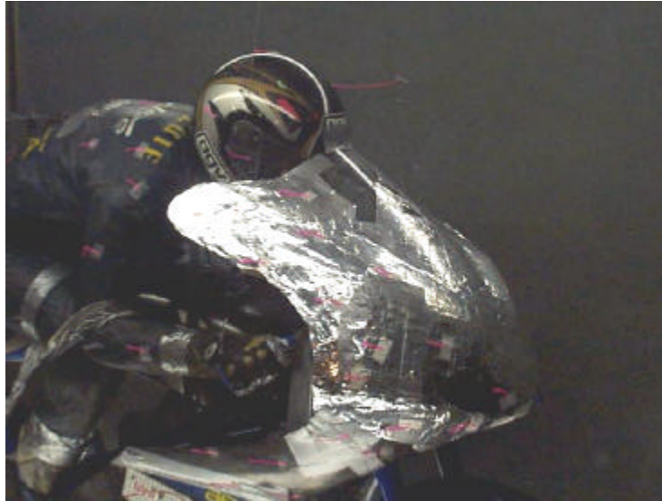
Figure 4.2: Final Shape of the Upper Fairing after Preliminary Testing.
