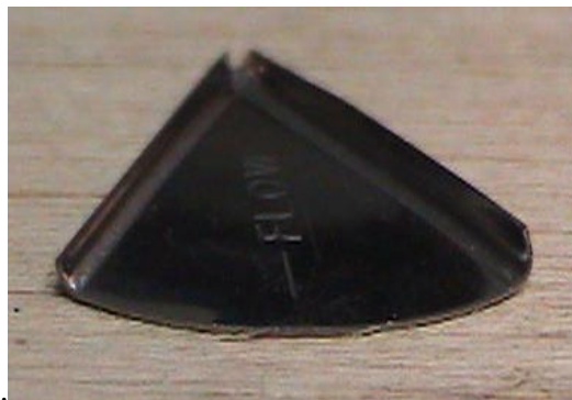
Figure 3.5: Modified 1/4-inch Vortex Generator. A. Front View B. Side View
