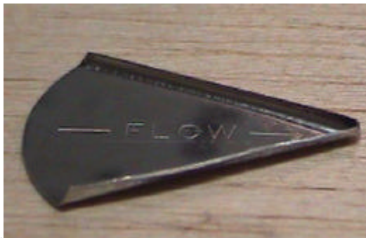
Figure 3.6: Modified 1/8-inch Vortex Generator. A. Top View B. Side View
