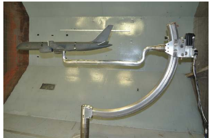
Figure 2.—3.5 percent Scale GTM installed in the NASA Langley 12-ft Low-Speed Wind Tunnel C-sector mounting and positioning system.
