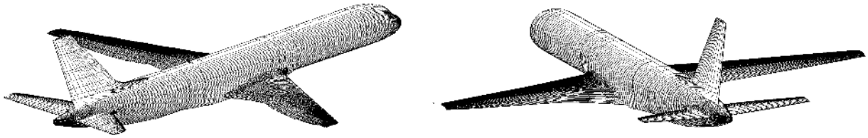
Figure 9. Example VCCTEF Deflected Wing Geometry
