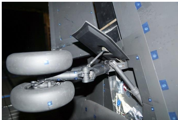
Figure 17. Frontal view of the 18% main landing gear without noise reduction concepts installed (baseline).
