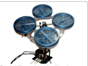
Figure 4 3-DOF hover simulation platform of the quad-rotor
