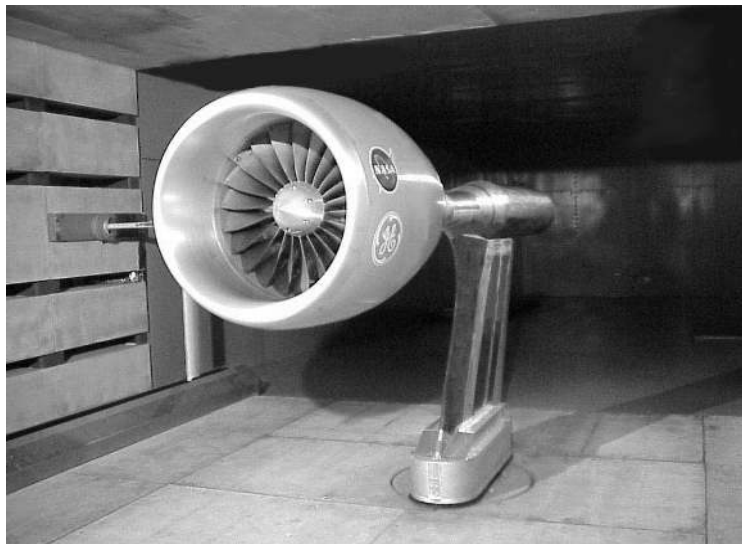
Figure 5. Fan module in the acoustic testing configuration installed on the UHB Drive Rig in the NASA Glenn 9- by 15-Foot Low Speed Wind Tunnel.
