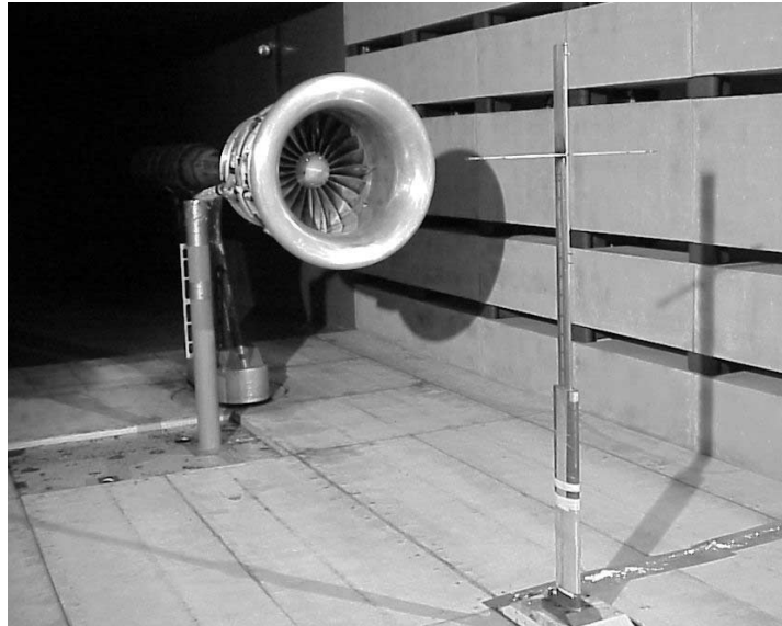
Figure 12. Fan module and freestream cruciform rake in the 9x15 during performance testing.
