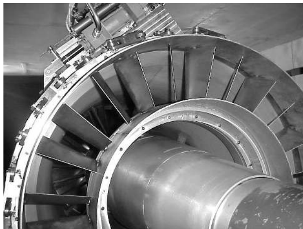
c. Close-up view of the VFEN installation on the UHB Drive Rig.
