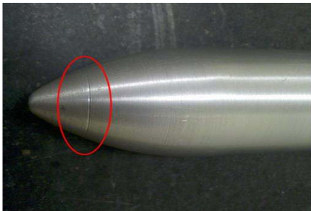
Figure 8. Machined Flaw on SLS-21000 Model
