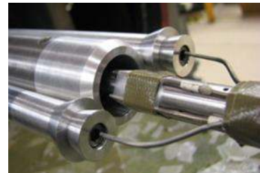
Figure 5. Base Pressure Tube Arrangement
