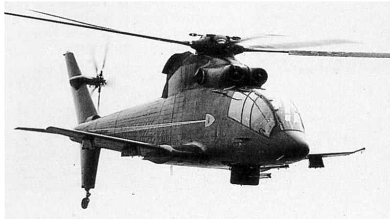
Figure 1.3 The Sikorsky S-67 Black Hawk, which is a lift compounded helicopter.
