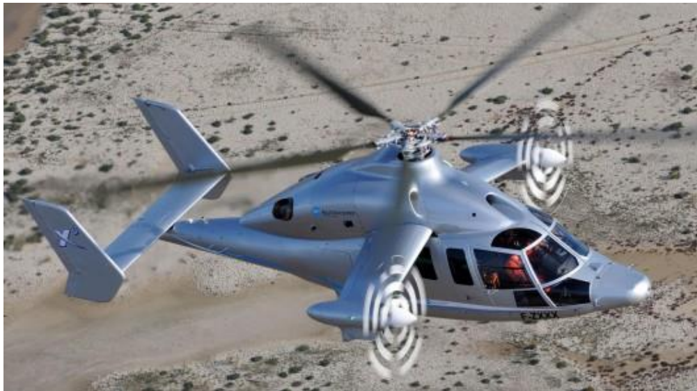
Figure 1.8 Airbus Helicopters X 3 , which is a lift and propulsive compounded helicopter.
