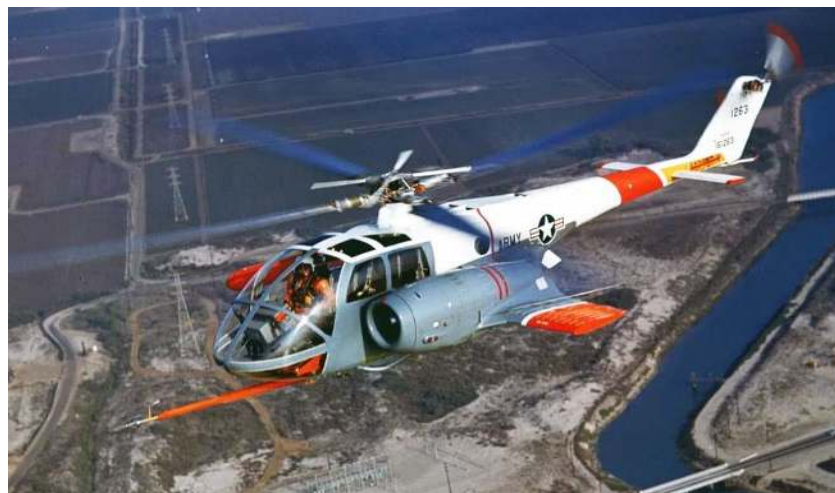
Figure 3.28 Lockheed XH-51 lift and propulsive compounded helicopter.
