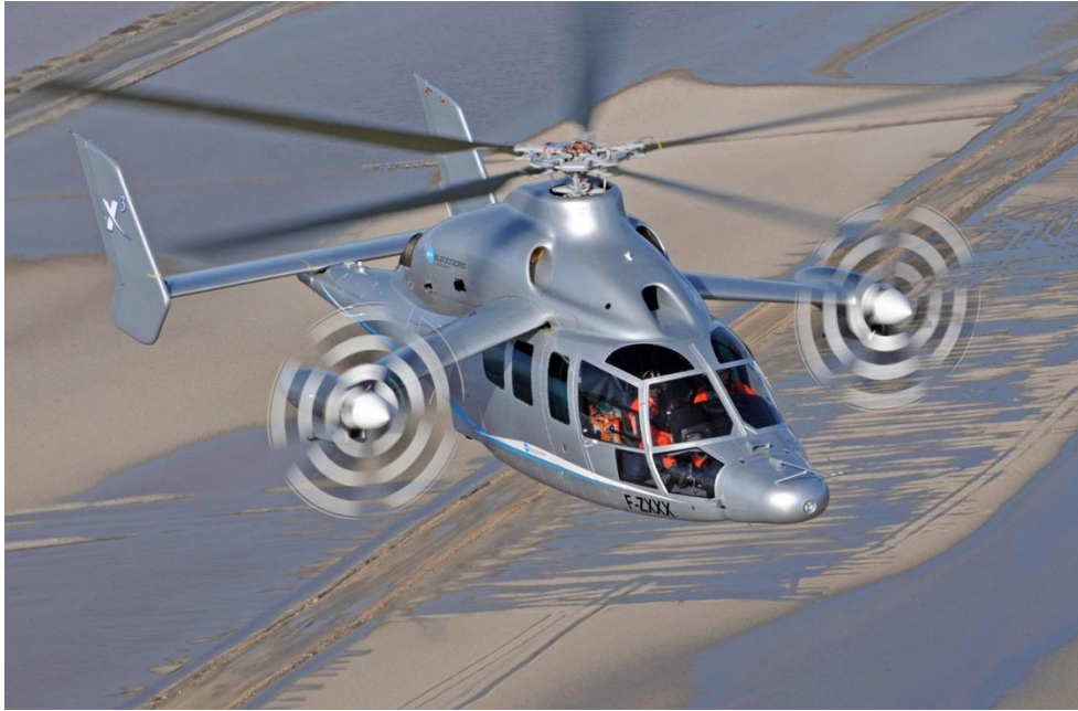
Figure 3.35 Airbus Helicopters X 3 , a lift and propulsive compounded helicopter.
