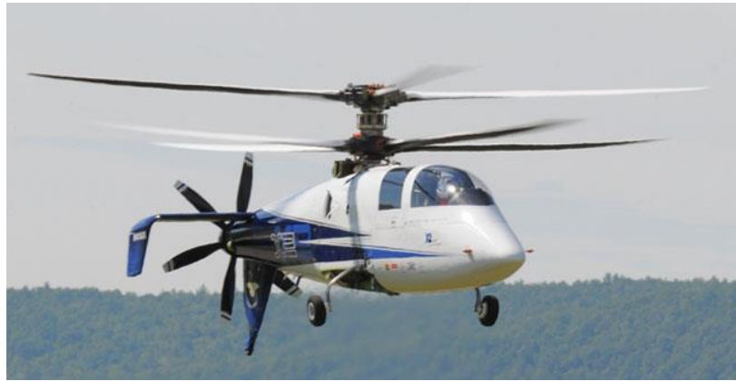
Figure 1.4 Sikorsky X2, which is a pure propulsive compounded helicopter.
