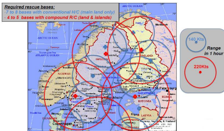
Figure 1.9 Medical bases required to cover northern Europe with a range of one hour for a conventional and compound helicopter (Cabrit, 2015).
