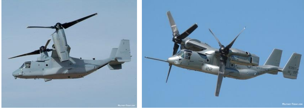
Figure 1.10 The V-22 Osprey at low airspeeds and in cruising flight configurations.
