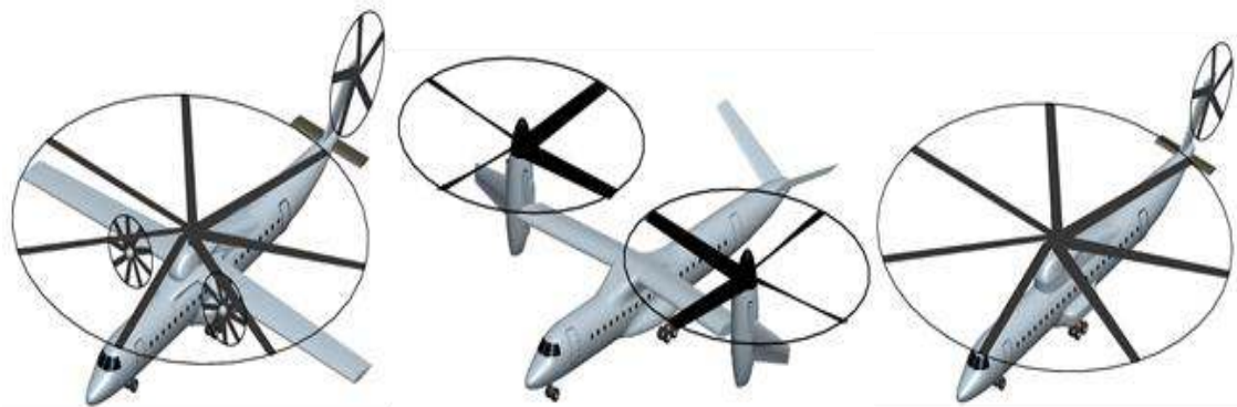
Figure 1.11 Compound, tiltrotor and conventional rotorcraft configurations studied by NASA (Johnson & Russel, 2012, pp. 5-7).
