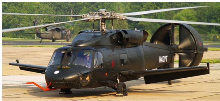
Figure 1.7 Piasecki X-49A, which is a lift and propulsive compounded helicopter.
