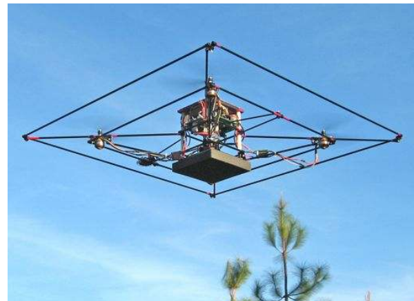
Fig. 1. The STARMAC II autonomous quadrotor helicopter in flight.
