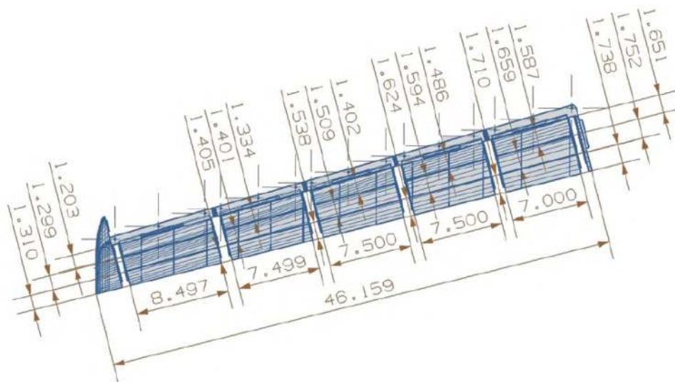
Drawing specifying planform view flap dimensions (measurements in inches)
