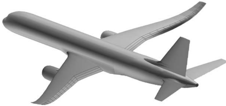
Figure 9 - Elastically Shaped Aircraft Concept with Variable Camber Continuous Trailing Edge Flap
