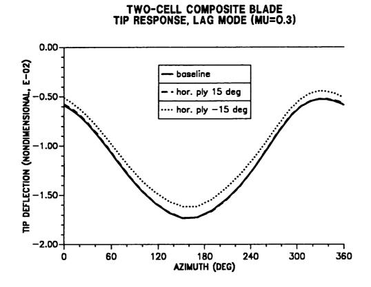
Figure 10.1: Effect of horizontal wall ply angle on blade tip response; lag mode ( $\mu = 0.30$ ).
