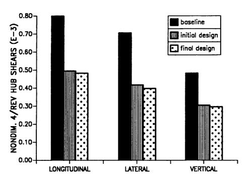
TWO-CELL COMPOSITE BLADE, SECOND CONFIGURATION OBJECTIVE FUNCTION J1 (MU=0.3)
