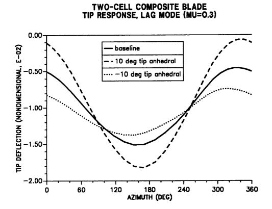
Figure 10.10: Effect of tip anhedral angle on blade tip response; lag mode  $(\mu = 0.30)$ .
