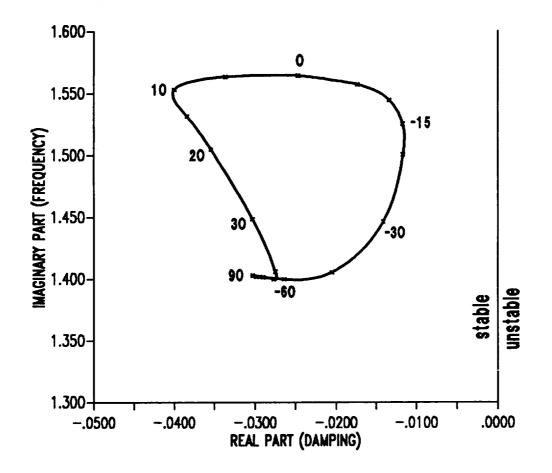
Figure 9.18: Root locus of first lag mode eigenvalues as a function of ply angle in horizontal wall for single-cell composite blade in hover.
