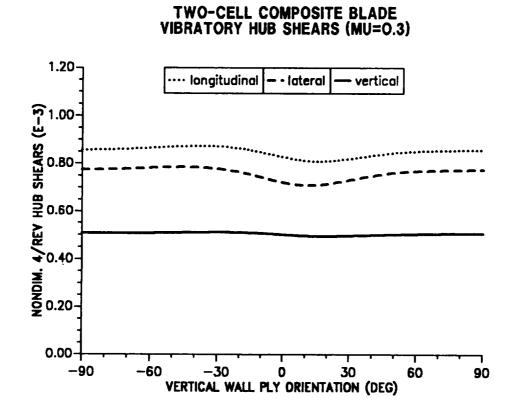
Figure 10.23: Effect of vertical wall ply angle on 4/rev hub shears  $(\mu = 0.30)$ .
