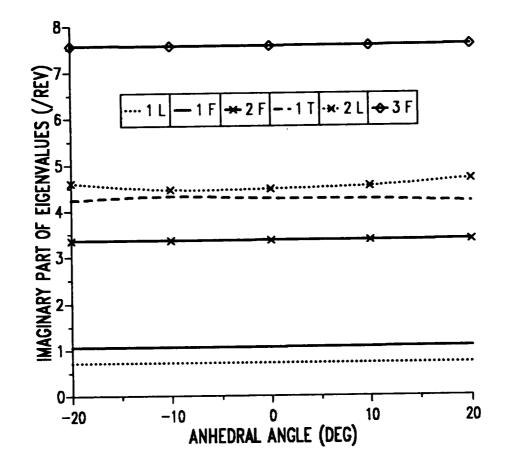
Figure 9.13: Effect of tip anhedral on the imaginary part of hover eigenvalues of isotropic blade, modified torsional frequency.
