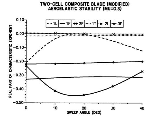
Figure 10.37: Effect of tip sweep angle on blade stability for the first six modes, modified torsional frequency ( $\mu = 0.30$ ).
