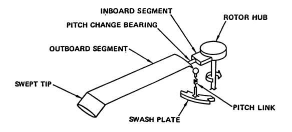
Figure 1.1: Rotor blade with tip sweep and anhedral
