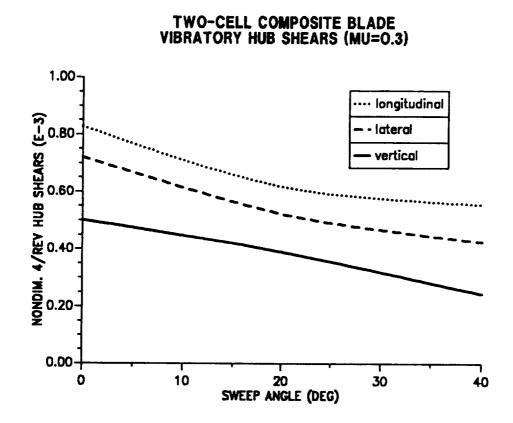
Figure 10.25: Effect of tip sweep angle on 4/rev hub shears ( $\mu = 0.30$ ).
