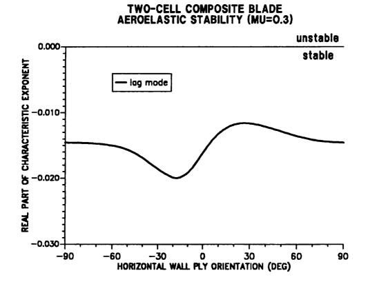
Figure 10.29: Effect of horizontal wall ply angle on blade stability; first lag mode ( $\mu = 0.30$ ).
