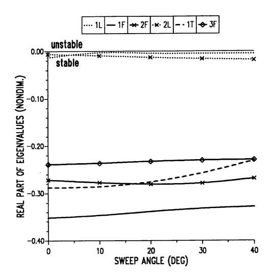
Figure 9.8: Effect of tip sweep on the real part of hover eigenvalues of isotropic blade, baseline configuration.
