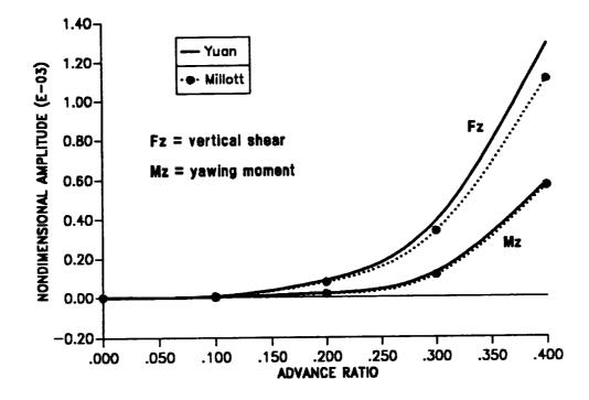
Figure 8.23: The 4/rev hub loads for soft-in-plane isotropic blade in forward flight; vertical shear and yawing moment.
