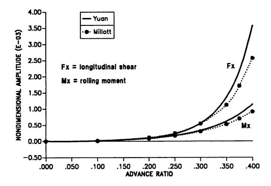
Figure 8.24: The 4/rev hub loads for stiff-in-plane isotropic blade in forward flight; logitudinal shear and rolling moment.
