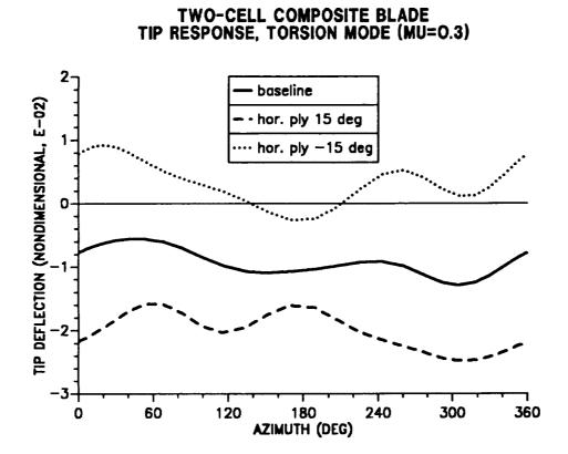
Figure 10.3: Effect of horizontal wall ply angle on blade tip response; torsion mode ( $\mu = 0.30$ ).
