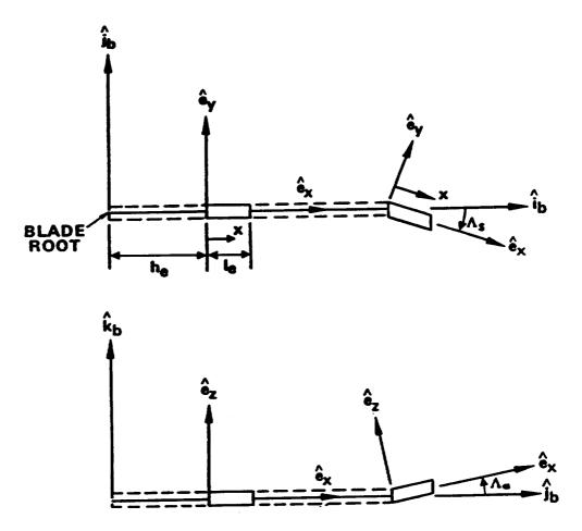
Figure 2.3: Undeformed element coordinate system
