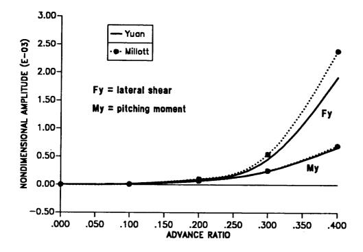
Figure 8.22: The 4/rev hub loads for soft-in-plane isotropic blade in forward flight; lateral shear and pitching moment.
