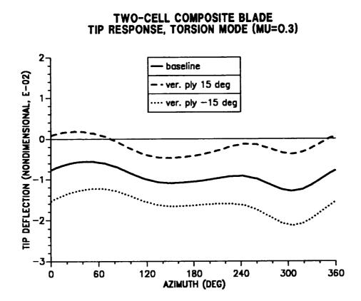
Figure 10.6: Effect of vertical wall ply angle on blade tip response; torsion mode ( $\mu = 0.30$ ).
