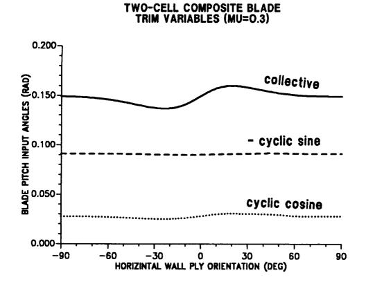
Figure 10.13: Effect of horizontal wall ply angle on trim variables; pitch setting ( $\mu = 0.30$ ).
