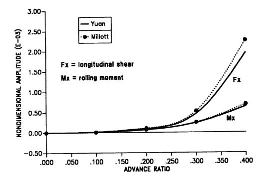
Figure 8.21: The 4/rev hub loads for soft-in-plane isotropic blade in forward flight; logitudinal shear and rolling moment.
