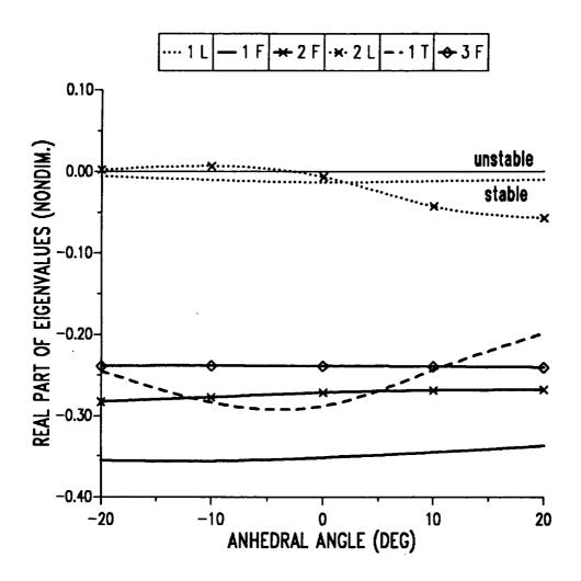
Figure 9.12: Effect of tip anhedral on the real part of hover eigenvalues of isotropic blade, baseline configuration.
