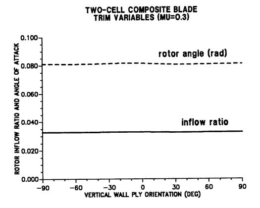
Figure 10.16: Effect of vertical wall ply angle on trim variables; inflow and rotor angle of attack ( $\mu = 0.30$ ).
