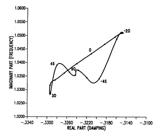
Figure 9.24: Root locus of first flap mode eigenvalues as a function of ply angle in vertical wall for two-cell composite blade in hover.
