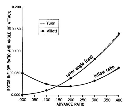
Figure 8.10: Trim variables for soft-in-plane isotropic blade in forward flight; inflow and rotor angle of attack.
