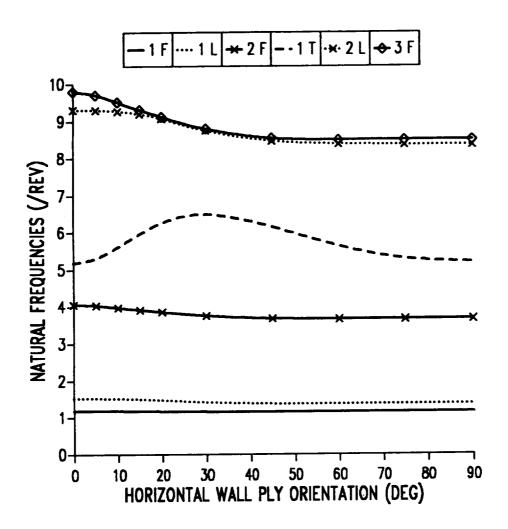
Figure 9.2: Natural frequencies as a function of ply angle in horizontal wall for single-cell composite blade.
