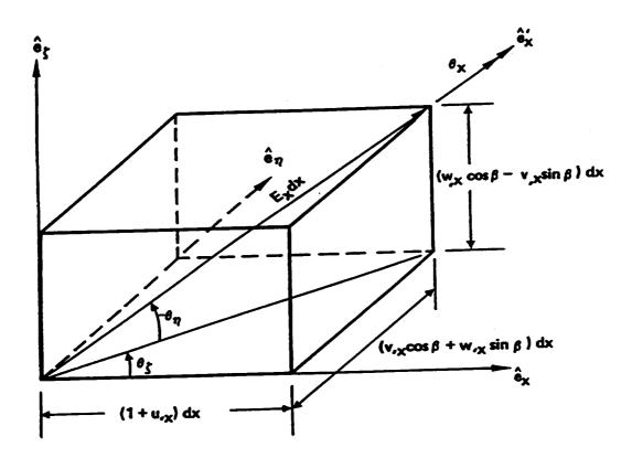
Figure 3.1: Deformation sequence and Euler angles
