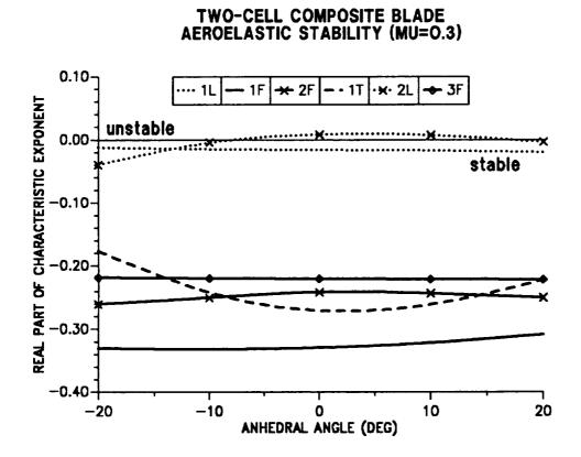
Figure 10.35: Effect of tip anhedral angle on blade stability for the first six modes ( $\mu = 0.30$ ).
