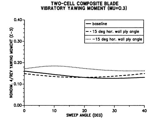
Figure 10.43: The 4/rev hub yawing moment as a function of tip sweep angle, combined effect with ply orientation ( $\mu = 0.30$ ).
