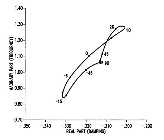
Figure 9.20: Root locus of first torsion mode eigenvalues as a function of ply angle in horizontal wall for single-cell composite blade in hover.
