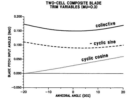
Figure 10.19: Effect of tip anhedral angle on trim variables; pitch setting  $(\mu = 0.30)$ .
