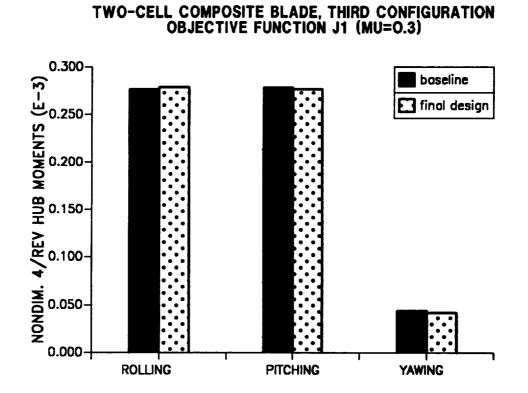
Figure 11.10: The 4/rev hub moments corresponding to third blade configuration (stiff-in-plane) and first objective function ( $\mu = 0.30$ ).
