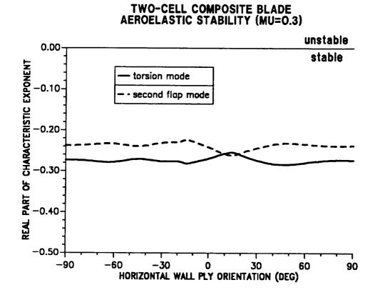
Figure 10.31: Effect of horizontal wall ply angle on blade stability; first torsion and second flap modes ( $\mu = 0.30$ ).
