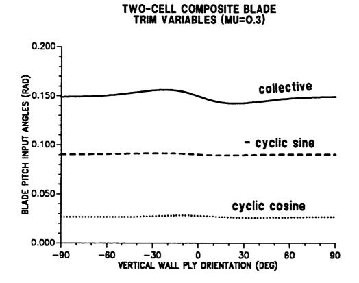
Figure 10.15: Effect of vertical wall ply angle on trim variables; pitch setting  $(\mu = 0.30)$ .
