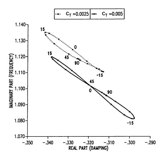
Figure 9.16: Root locus of first flap mode eigenvalues as a function of ply angle in vertical wall for single-cell composite blade in hover.
