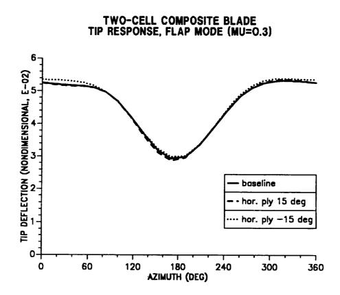
Figure 10.2: Effect of horizontal wall ply angle on blade tip response; flap mode ( $\mu = 0.30$ ).
