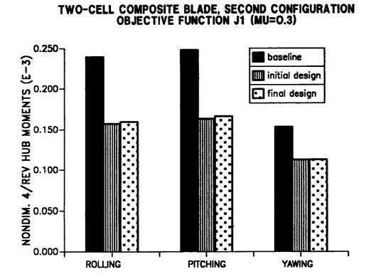
Figure 11.6: The 4/rev hub moments corresponding to second blade configuration (soft-in-plane) and first objective function ( $\mu = 0.30$ ).
