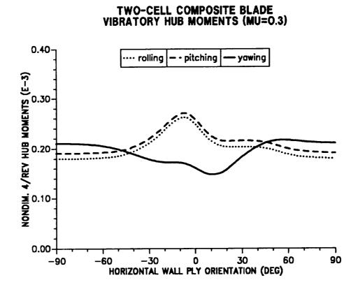
Figure 10.22: Effect of horizontal wall ply angle on 4/rev hub moments  $(\mu = 0.30)$ .
