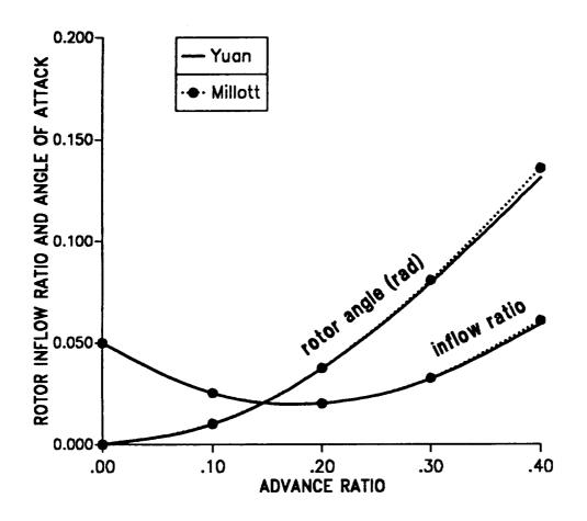
Figure 8.12: Trim variables for stiff-in-plane isotropic blade in forward flight; inflow and rotor angle of attack.
