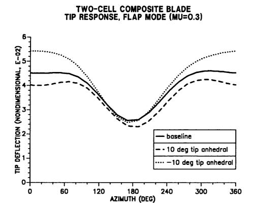
Figure 10.11: Effect of tip anhedral angle on blade tip response; flap mode  $(\mu = 0.30)$ .
