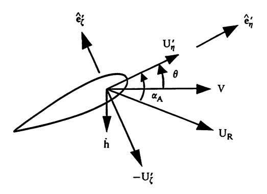
Figure 5.1: Components of blade velocity relative to the air
