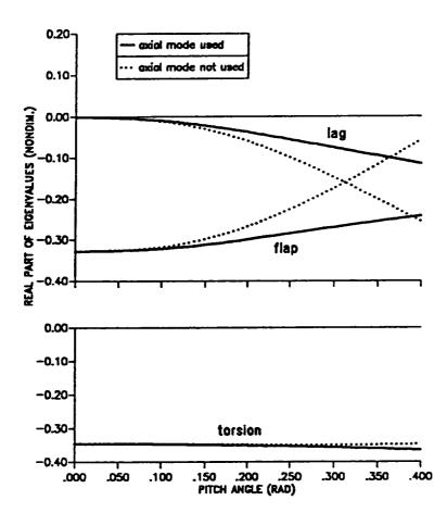
Figure 8.6: Effect of axial mode on the real part of hover eigenvalues of isotropic blade. Analysis with substitution.
