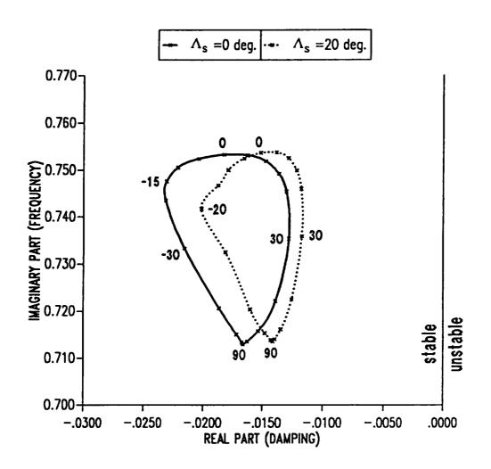
Figure 9.26: Root locus of first lag mode eigenvalues as a function of ply angle in horizontal wall for two-cell composite blade in hover.
