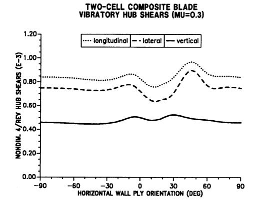
Figure 10.21: Effect of horizontal wall ply angle on 4/rev hub shears  $(\mu = 0.30)$ .
