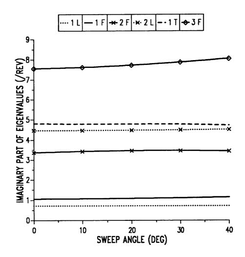
Figure 9.7: Effect of tip sweep on the imaginary part of hover eigenvalues of isotropic blade, baseline configuration.
