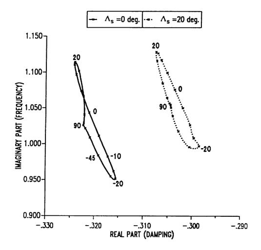
Figure 9.27: Root locus of first flap mode eigenvalues as a function of ply angle in horizontal wall for two-cell composite blade in hover.
