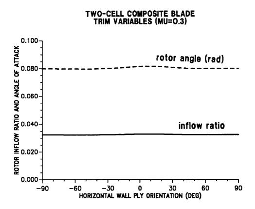
Figure 10.14: Effect of horizontal wall ply angle on trim variables; inflow and rotor angle of attack ( $\mu = 0.30$ ).
