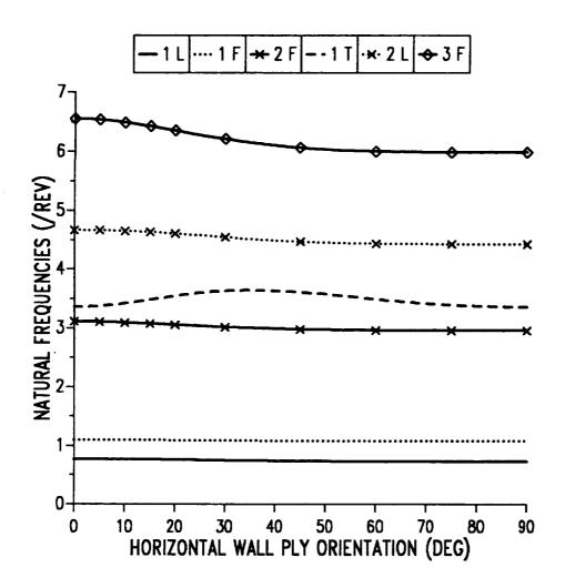
Figure 9.4: Natural frequencies as a function of ply angle in horizontal wall for two-cell composite blade.
