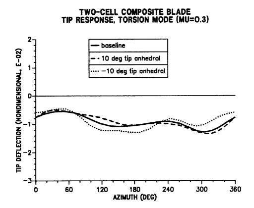
Figure 10.12: Effect of tip anhedral angle on blade tip response; torsion mode ( $\mu = 0.30$ ).
