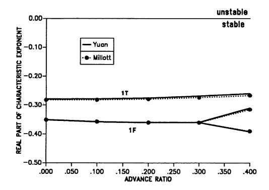
Figure 8.16: Blade damping for soft-in-plane isotropic blade in forward flight; first flap and torsion modes.
