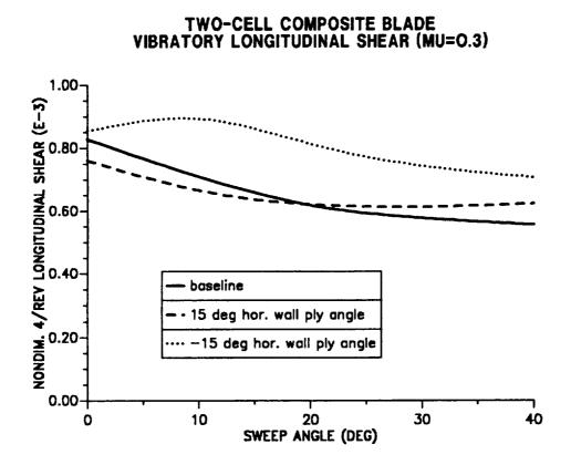
Figure 10.38: The 4/rev longitudinal hub shear as a function of tip sweep angle, combined effect with ply orientation ( $\mu = 0.30$ ).
