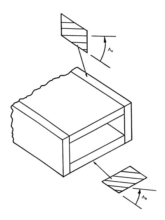
Figure 8.7: Single-cell composite rectangular box beam
