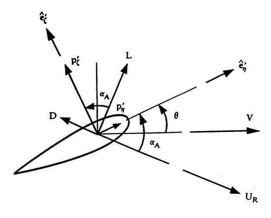
Figure 5.2: Components of acrodynamic force acting on the blade
