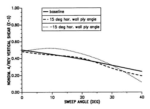
Figure 10.40: The 4/rev vertical hub shear as a function of tip sweep angle, combined effect with ply orientation ( $\mu = 0.30$ ).
