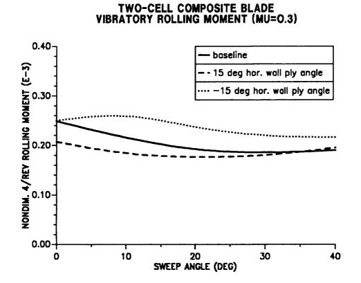
Figure 10.41: The 4/rev hub rolling moment as a function of tip sweep angle, combined effect with ply orientation ( $\mu = 0.30$ ).
