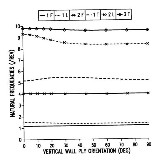
Figure 9.1: Natural frequencies as a function of ply angle in vertical wall for single-cell composite blade.
