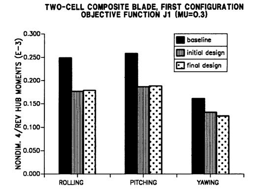
Figure 11.2: The 4/rev hub moments corresponding to first blade configuration (soft-in-plane) and first objective function ( $\mu = 0.30$ ).
