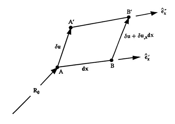
Figure 4.1: Motion of an element on the deformed elastic axis during the virtual displacement
