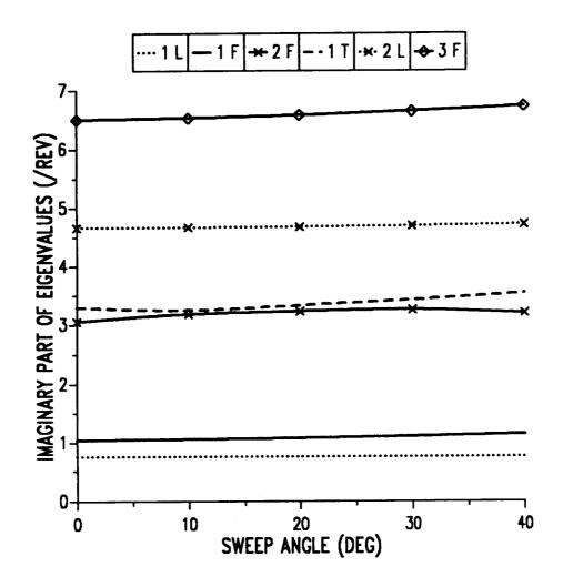
Figure 9.21: Effect of tip sweep on the imaginary part of hover eigenvalues of two-cell composite blade, baseline configuration.
