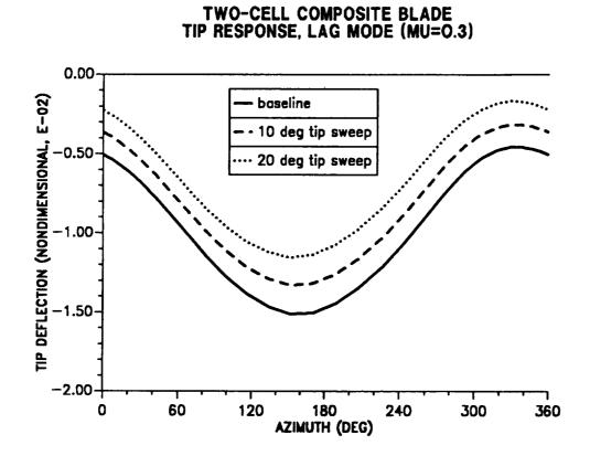
Figure 10.7: Effect of tip sweep angle on blade tip response; lag mode  $(\mu = 0.30)$ .
