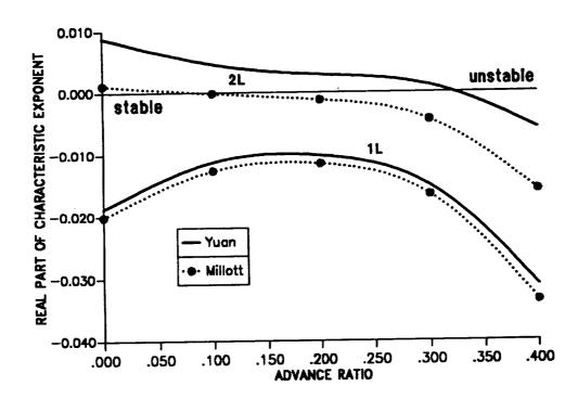
Figure 8.15: Blade damping for soft-in-plane isotropic blade in forward flight; first and second lag modes.
