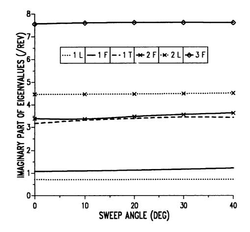
Figure 9.9: Effect of tip sweep on the imaginary part of hover eigenvalues of isotropic blade, modified torsional frequency.
