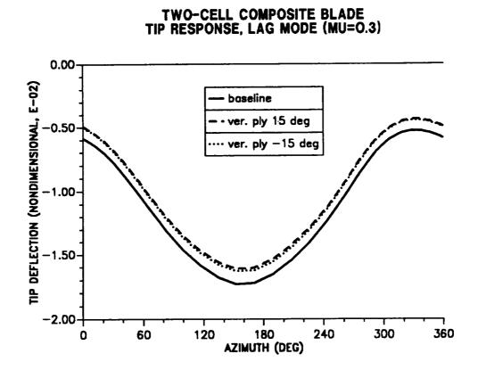
Figure 10.4: Effect of vertical wall ply angle on blade tip response; lag mode  $(\mu = 0.30)$ .
