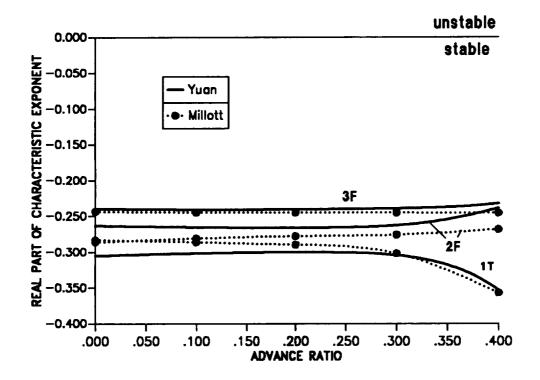
Figure 8.20: Blade damping for stiff-in-plane isotropic blade in forward flight; first torsion, second and third flap modes.
