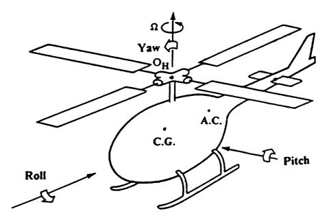
Figure 6.1: Schematic of a four-bladed helicopter
