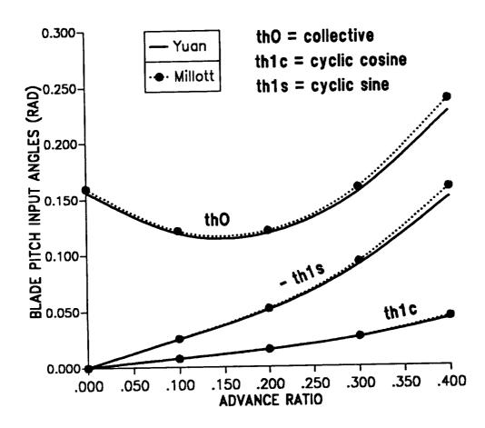
Figure 8.9: Trim variables for soft-in-plane isotropic blade in forward flight; pitch setting.
