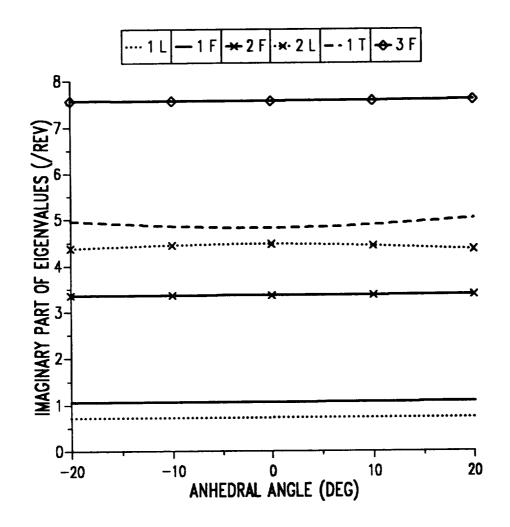
Figure 9.11: Effect of tip anhedral on the imaginary part of hover eigenvalues of isotropic blade, baseline configuration.
