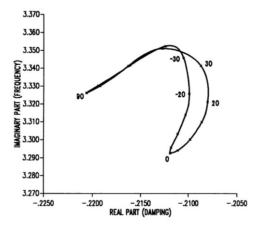
Figure 9.25: Root locus of first torsion mode eigenvalues as a function of ply angle in vertical wall for two-cell composite blade in hover.
