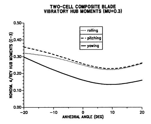
Figure 10.28: Effect of tip anhedral angle on 4/rev hub moments ( $\mu = 0.30$ ).
