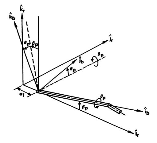
Figure 2.2: Preconed, pitched, blade-fixed coordinate system
