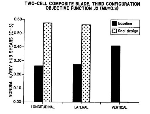
Figure 11.11: The 4/rev hub shears corresponding to third blade configuration (stiff-in-plane) and second objective function ( $\mu = 0.30$ ).
