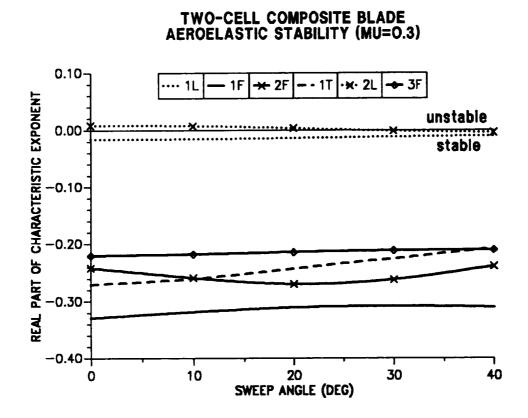
Figure 10.34: Effect of tip sweep angle on blade stability for the first six modes ( $\mu = 0.30$ ).
