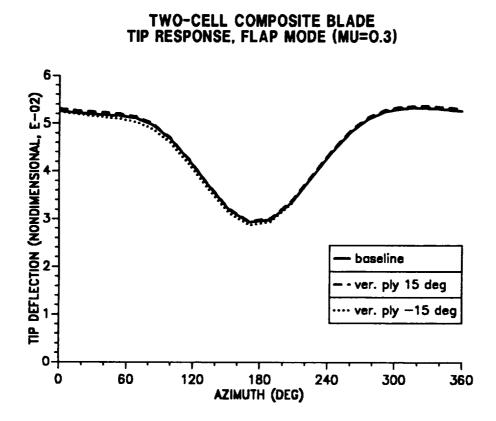
Figure 10.5: Effect of vertical wall ply angle on blade tip response; flap mode  $(\mu = 0.30)$ .
