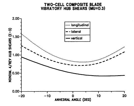
Figure 10.27: Effect of tip anhedral angle on 4/rev hub shears ( $\mu = 0.30$ ).
