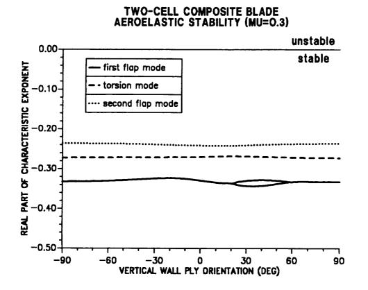
Figure 10.33: Effect of vertical wall ply angle on blade stability; first, second flap and first torsion modes ( $\mu = 0.30$ ).
