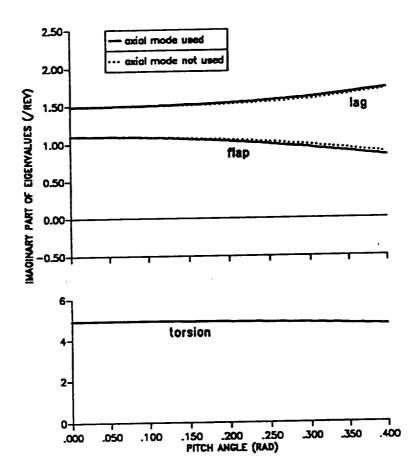
Figure 8.5: Effect of axial mode on the imaginary part of hover eigenvalues of isotropic blade. Analysis with substitution.
