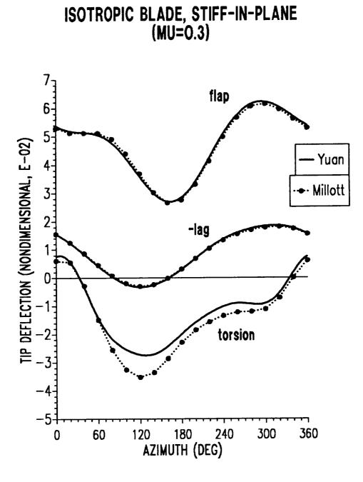
Figure 8.14: Blade tip response for stiff-in-plane isotropic blade ( $\mu = 0.30$ ).
