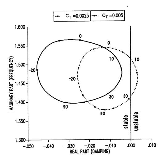
Figure 9.15: Root locus of first lag mode eigenvalues as a function of ply angle in vertical wall for single-cell composite blade in hover.
