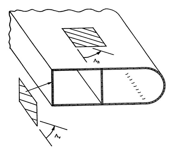
Figure 7.1: Finite element model for two-cell composite cross section
