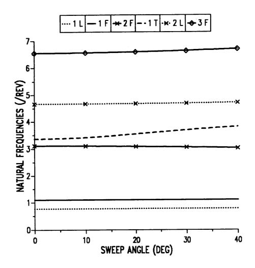
Figure 9.5: Natural frequencies as a function of tip sweep angle for two-cell composite blade with zero ply angle.
