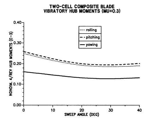
Figure 10.26: Effect of tip sweep angle on 4/rev hub moments ( $\mu = 0.30$ ).
