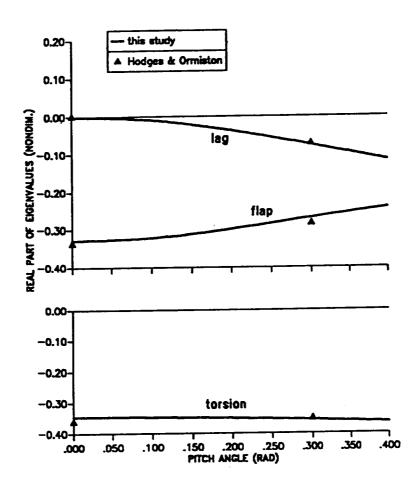
Figure 8.3: Real part of hover eigenvalues of isotropic blade, as a function of blade collective pitch.
