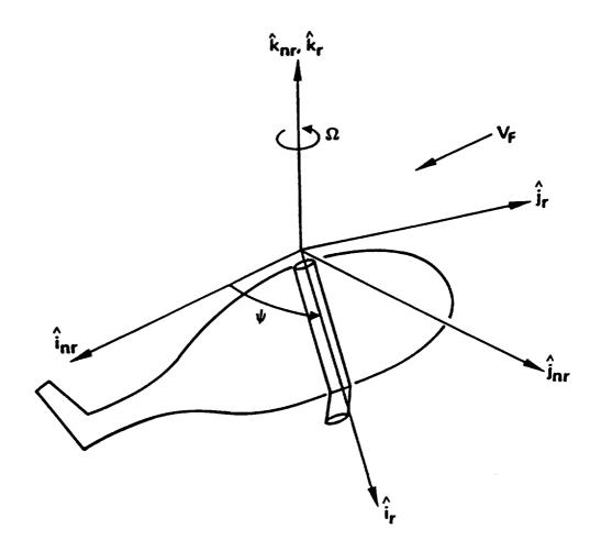
Figure 2.1: Nonrotating, hub-fixed coordinate system and rotating, hub-fixed coordinate system
