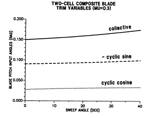
Figure 10.17: Effect of tip sweep angle on trim variables; pitch setting  $(\mu = 0.30)$ .
