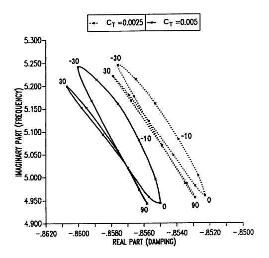
Figure 9.17: Root locus of first torsion mode eigenvalues as a function of ply angle in vertical wall for single-cell composite blade in hover.
