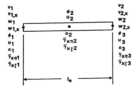
Figure 4.2: Finite element nodal degrees of freedom
