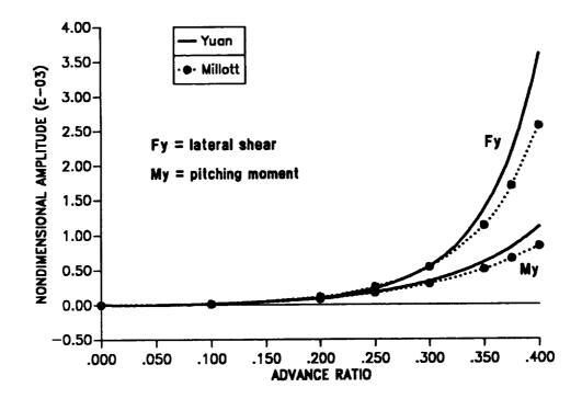
Figure 8.25: The 4/rev hub loads for stiff-in-plane isotropic blade in forward flight; lateral shear and pitching moment.
