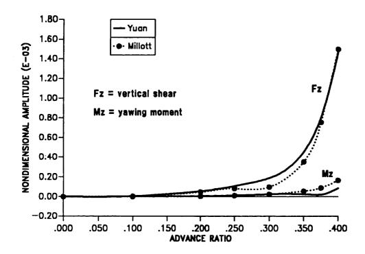
Figure 8.26: The 4/rev hub loads for stiff-in-plane isotropic blade in forward flight; vertical shear and yawing moment.
