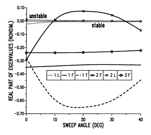
Figure 9.10: Effect of tip sweep on the real part of hover eigenvalues of isotropic blade, modified torsional frequency.
