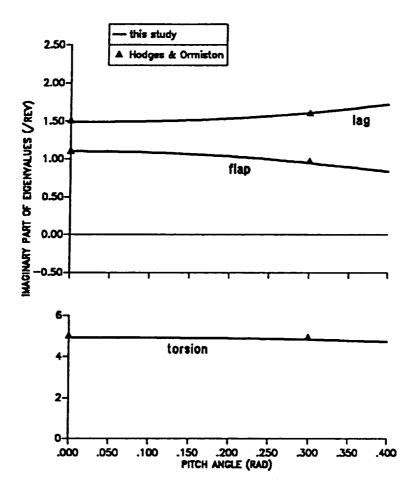
Figure 8.2: Imaginary part of hover eigenvalues of isotropic blade, as a function of blade collective pitch.
