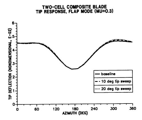
Figure 10.8: Effect of tip sweep angle on blade tip response; flap mode  $(\mu = 0.30)$ .
