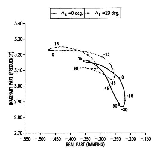
Figure 9.29: Root locus of second flap mode eigenvalues as a function of ply angle in horizontal wall for two-cell composite blade in hover.
