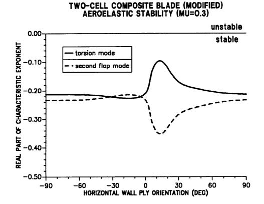
Figure 10.36: Effect of horizontal wall ply angle on stability of first torsion and second flap modes, modified torsional frequency  $(\mu = 0.30)$ .
