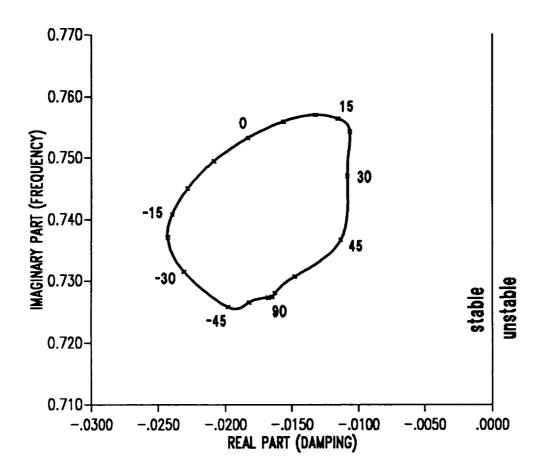
Figure 9.23: Root locus of first lag mode eigenvalues as a function of ply angle in vertical wall for two-cell composite blade in hover.
