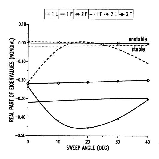
Figure 9.22: Effect of tip sweep on the real part of hover eigenvalues of two-cell composite blade, baseline configuration.
