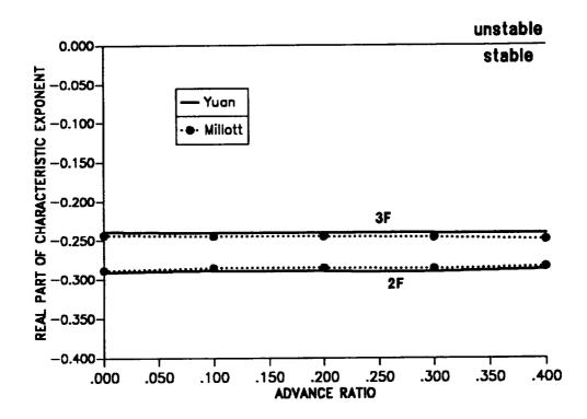
Figure 8.17: Blade damping for soft-in-plane isotropic blade in forward flight; second and third flap modes.
