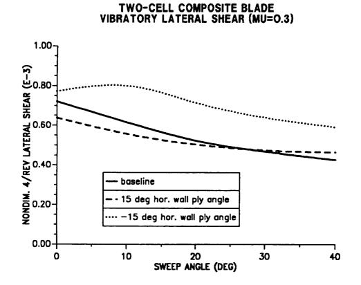
Figure 10.39: The 4/rev lateral hub shear as a function of tip sweep angle, combined effect with ply orientation ( $\mu = 0.30$ ).
