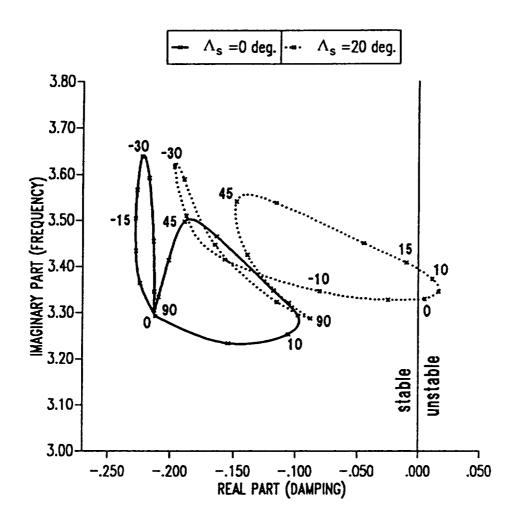
Figure 9.28: Root locus of first torsion mode eigenvalues as a function of ply angle in horizontal wall for two-cell composite blade in hover.
