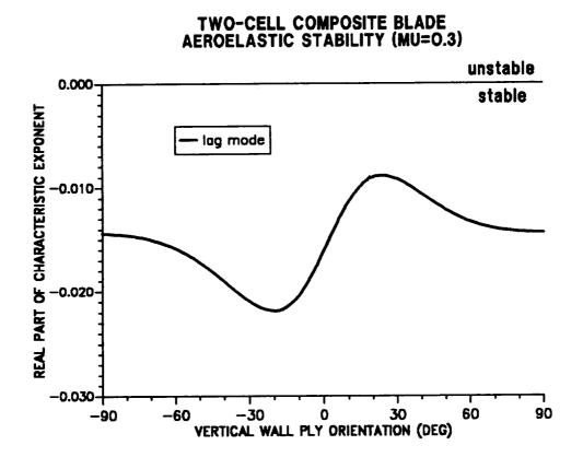
Figure 10.32: Effect of vertical wall ply angle on blade stability; first lag mode ( $\mu = 0.30$ ).
