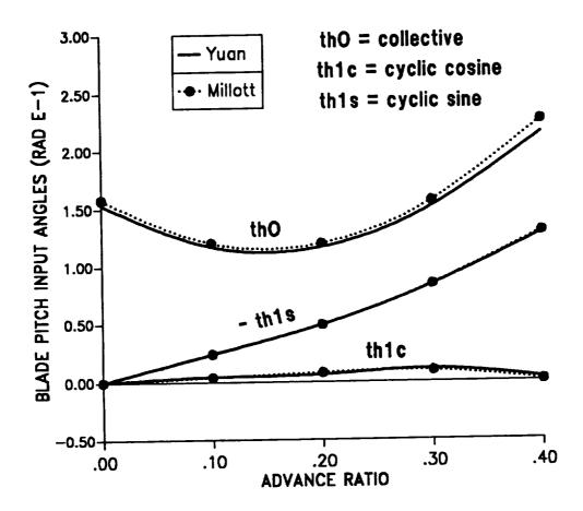
Figure 8.11: Trim variables for stiff-in-plane isotropic blade in forward flight; pitch setting.
