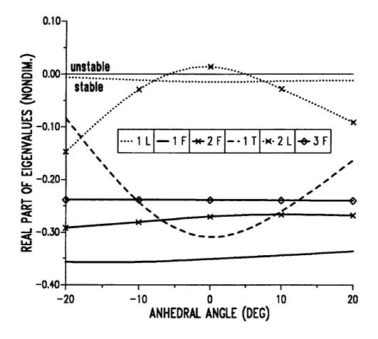
Figure 9.14: Effect of tip anhedral on the real part of hover eigenvalues of isotropic blade, modified torsional frequency.
