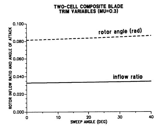
Figure 10.18: Effect of tip sweep angle on trim variables; inflow and rotor angle of attack ( $\mu = 0.30$ ).
