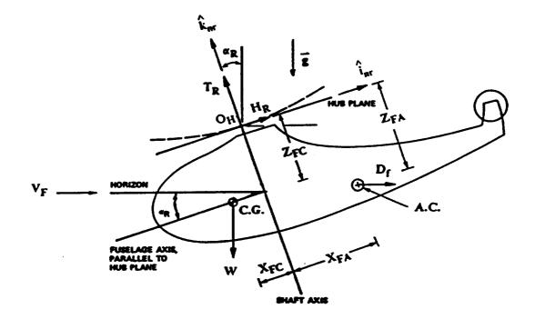
Figure 6.2: Forces on the helicopter in steady, level flight
