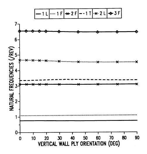
Figure 9.3: Natural frequencies as a function of ply angle in vertical wall for two-cell composite blade.
