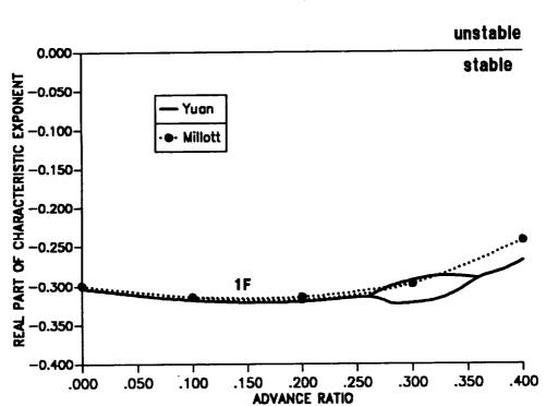
Figure 8.19: Blade damping for stiff-in-plane isotropic blade in forward flight; first flap mode.
