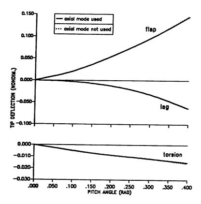
Figure 8.4: Effect of axial mode on the nonlinear equilibrium position of isotropic blade in hover. Analysis with substitution.
