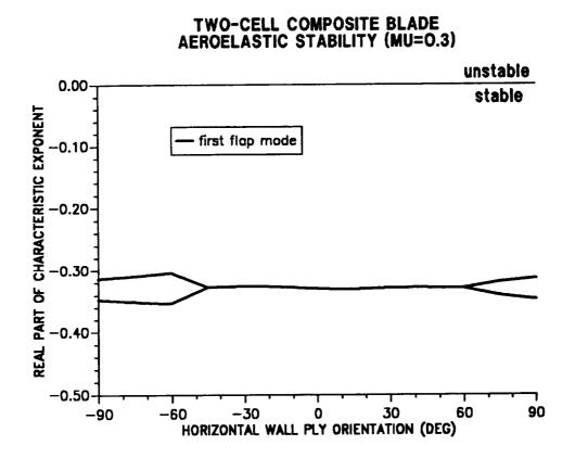
Figure 10.30: Effect of horizontal wall ply angle on blade stability; first flap mode ( $\mu = 0.30$ ).
