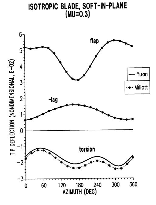
Figure 8.13: Blade tip response for soft-in-plane isotropic blade ( $\mu = 0.30$ ).
