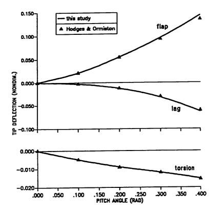
Figure 8.1: Nonlinear equilibrium position of isotropic blade in hover, as a function of blade collective pitch.
