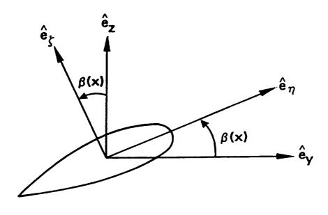
Figure 2.4: Undeformed curvilinear coordinate system
