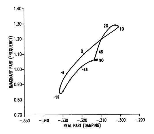
Figure 9.19: Root locus of first flap mode eigenvalues as a function of ply angle in horizontal wall for single-cell composite blade in hover.
