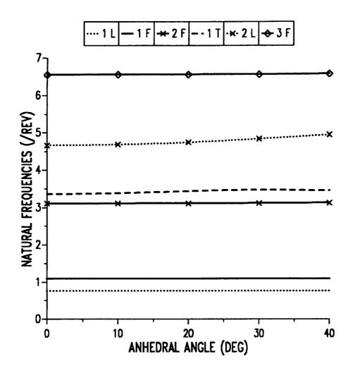
Figure 9.6: Natural frequencies as a function of tip anhedral angle for twocell composite blade with zero ply angle.
