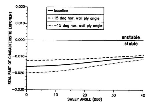
Figure 10.44: Real part of characteristic exponent of blade first lag mode as a function of tip sweep angle, combined effect with ply orientation ( $\mu = 0.30$ ).
