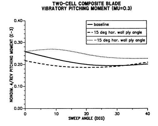
Figure 10.42: The 4/rev hub pitching moment as a function of tip sweep angle, combined effect with ply orientation ( $\mu = 0.30$ ).
