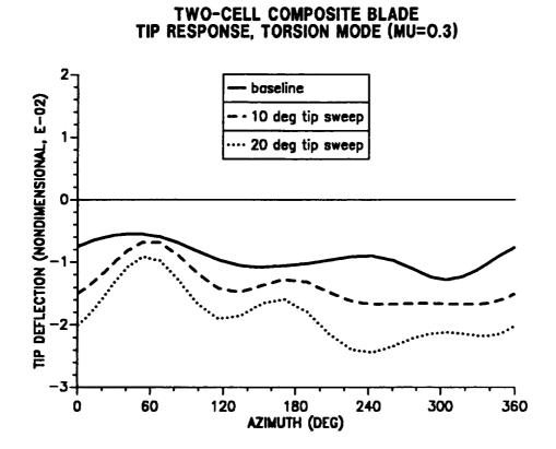
Figure 10.9: Effect of tip sweep angle on blade tip response; torsion mode  $(\mu = 0.30)$ .
