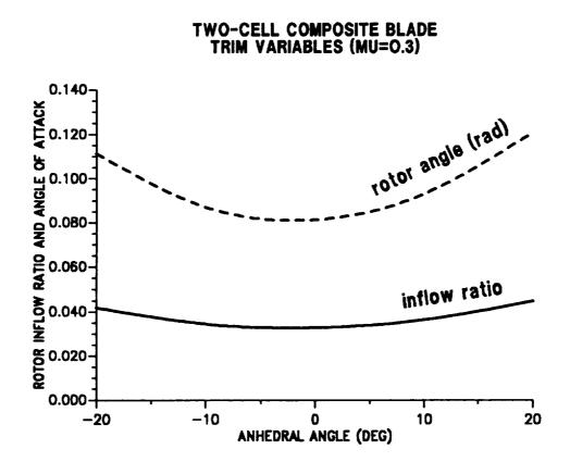
Figure 10.20: Effect of tip anhedral angle on trim variables; inflow and rotor angle of attack ( $\mu = 0.30$ ).
