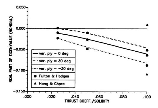
Figure 8.8: Real part of hover eigenvalues for single-cell composite blade as a function of (thrust coefficient/solidity).
