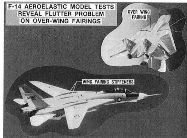
Figure 14. F-14 aeroelastic model tests revealed flutter problem on over-wing fairing.
