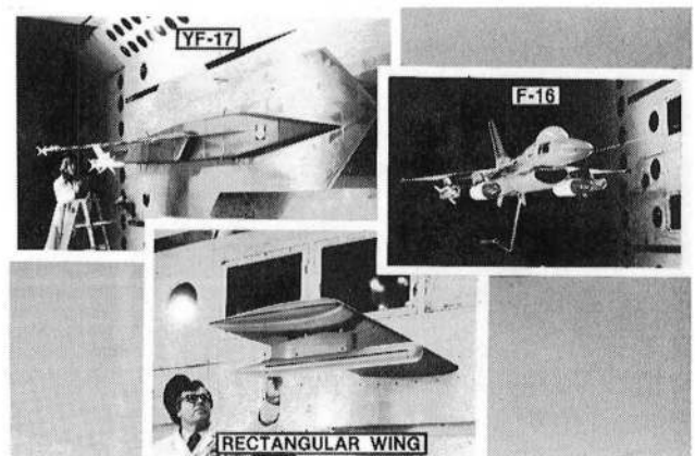
Figure 19. Wing/store flutter suppression studies in the Langley TDT.
