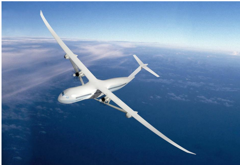
Fig. 1 - Boeing SUGAR Truss-Braced Wing (TBW) Aircraft Concept
