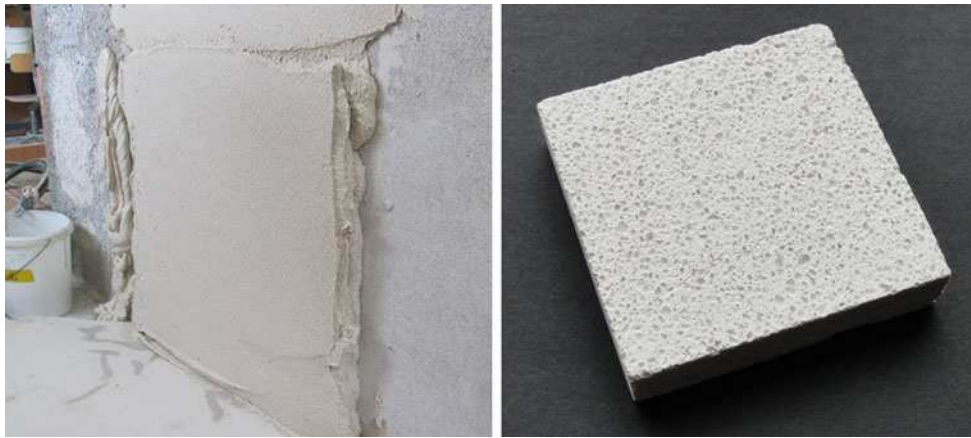
Fig. 21 High-performance insulating render system developed by Empa and Fixit. Wall spray test ( left ) and cut cross section of the material clearly showing individual aerogel granules ( right )
