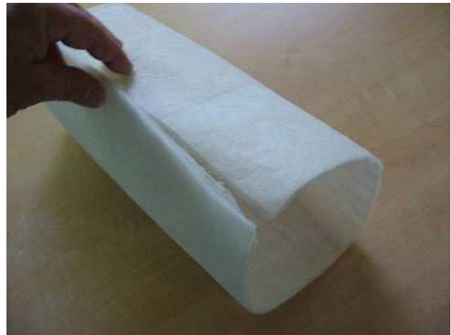
Fig. 15 Photograph of the ambient-dried silica aerogel-based blanket observed in Fig. 14, with courtesy of. Bonnardel P.A, PCAS, Longjumeau, France and Sallée H. CSTB, Grenoble, France
