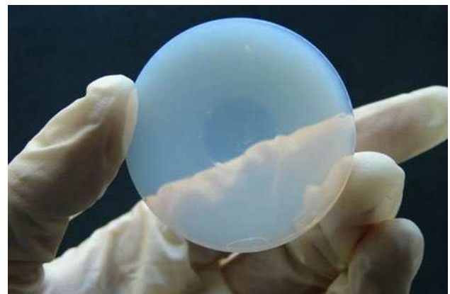
Fig. 11 Example of silica aerogel monolith (sample synthesized by a two-step catalytic process from TEOS and dried with supercritical \text{CO}_2 , presenting a density of 0.13 \text{ g cm}^{-3} and an effective thermal conductivity of 0.015 \text{ Wm}^{-1} \text{ K}^{-1} as respectively measured by mercury pycnometry and with the hot-wire method at room temperature)
