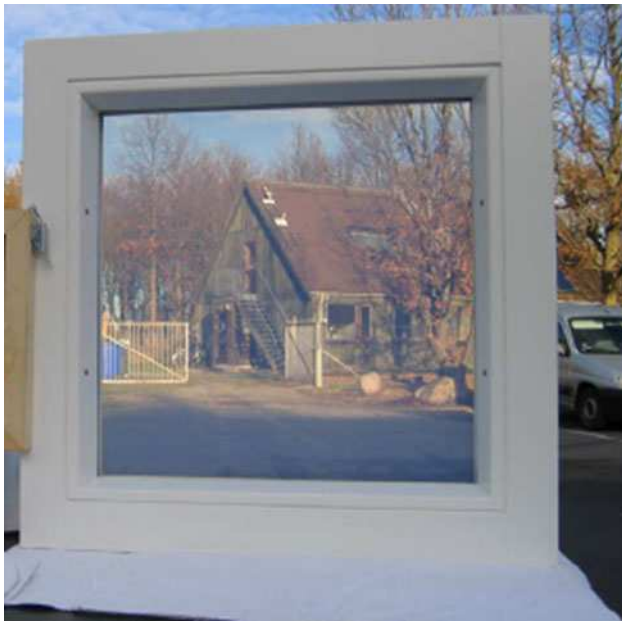
Fig. 18 Example of super-insulating aerogel glazings developed within the frame of the HILIT+ European project based on the use of silica aerogels plates from AIRGLASS AB (inspired from [122])
