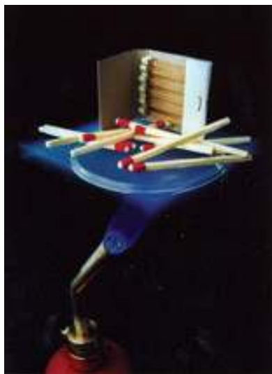
FIGURE 1: Matches on aerogel over a flame [17].
