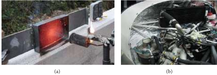
FIGURE 7: Aerogel firewall during testing. (Image courtesy Aspen Aerogel). Pyrogel 6350 installed in aircraft engine for fire protection (Image courtesy Aspen Aerogel).
