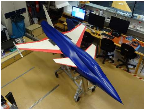
Figure 10. The generic fighter aeroelastic wind-tunnel model tested in summer of 2016.
