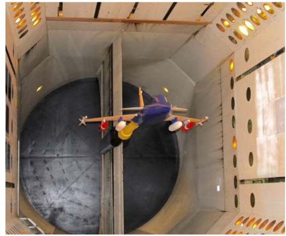
Figure 11. The generic fighter aeroelastic wind-tunnel model installed in the Transonic Dynamics Tunnel (TDT).
