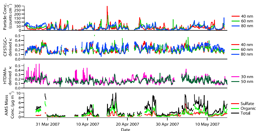
Fig. 4. Temporal variation of HTDMA-derived and CCN-derived \kappa values, total particle concentration, and AMS mass concentration throughout the campaign.
