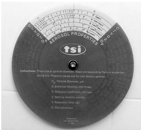
(B) Aerosol Properties Slide Rule—1981
