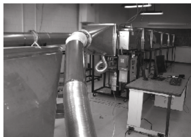
Figure 37. Bioaerosol test facility based on American Society of Heating, Refrigerating and Air-Conditioning Engineers (ASHRAE) Standard 52.2, 2004.
