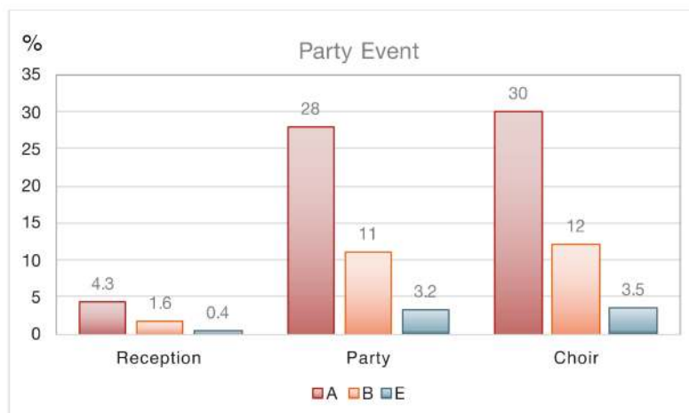
Figure 2. Individual risk of a particular person being infected (equivalent to the percentage of the group being infected), comparing a party with a reception and a choir practice, for three scenarios. Scenario A: passive ventilation, no masks. Scenario B: active ventilation with outside air, no masks. Scenario E: High-volume filtration with HEPA.
