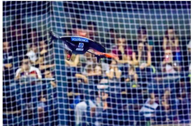
Fig. 1: Parrot ARDrone 2 carrying out a fully autonomous emulated indoors search and rescue mission during an exhibition in the European Night of the Researchers (described in section IV) in front of an audience of 400 people using Aerostack. No Motion Capture System is used.
