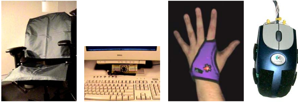
Fig 1 Various sensors can capture postural, facial, skin-surface, and gestural changes that carry affective information. From left to right: chair with Tekscan pressure sensors, BlueEyes camera, Galvactivator skin conductivity sensor, and pressure mouse.
