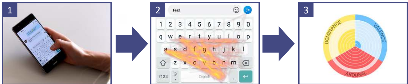
Figure 1. Our system extracts touch input characteristics of users while typing on smartphones (1) and aggregates these metrics into two-dimensional heat maps (2). A semi-supervised classification pipeline dynamically predicts affective states (valence, arousal, and dominance) of the user (3).
