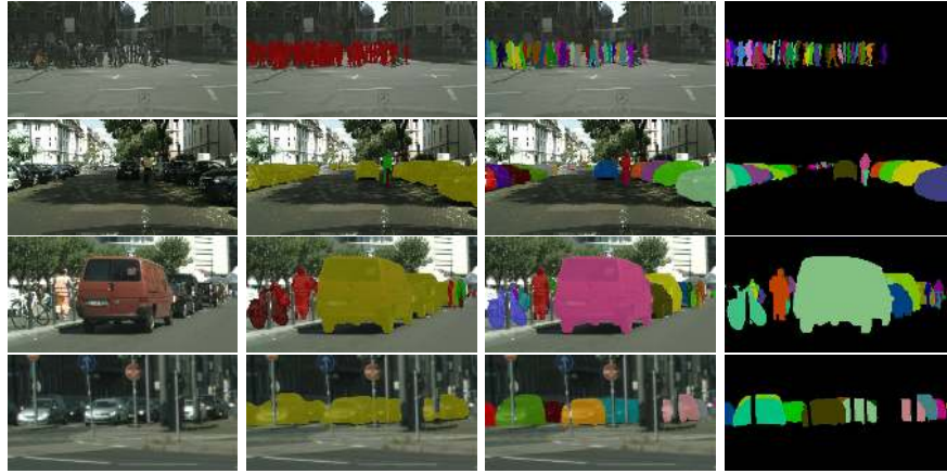
Fig. 6. Results on Cityscapes val dataset, original image, semantic results, instance results and ground truth from left to right. Results in the last two rows are cropped from the original ones for better visualization.
