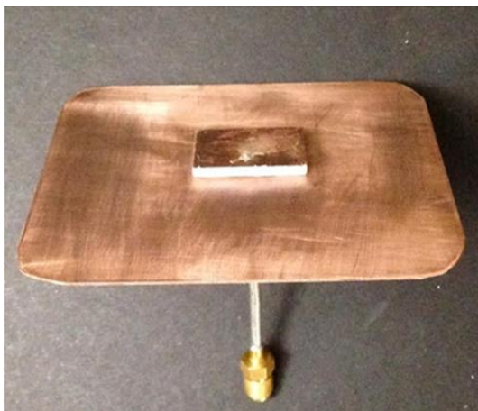
Figure 2. Fabricated and metalized 3D printed Patch Antenna. b. Logo Patch Antenna (Spartan block 'S')
