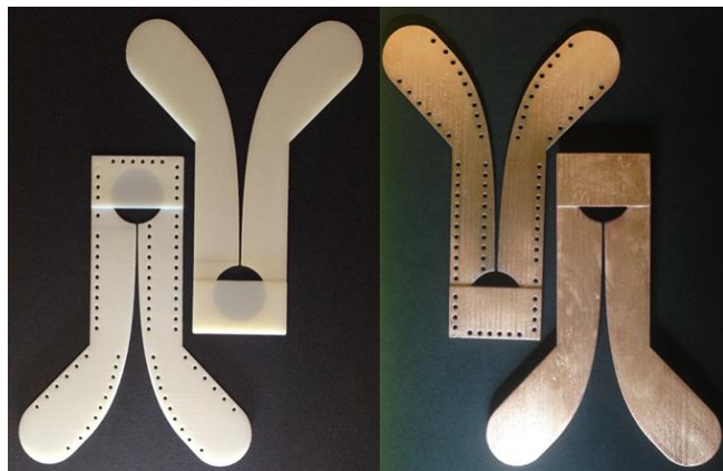
Figure 17. Fabricated 3D printed Bilateral Vivaldi Antenna before and after metallization, prior to assembly.
