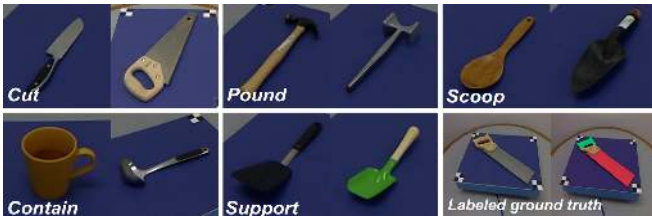
Fig. 4: Sample objects from the RGB-D Part Affordance Dataset. (Lower-right) An example of a full frame image with hand-labeled ground truth. The ground truth labels include rankings for multiple affordances.
