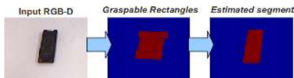
Fig. 6: Estimating pixel accurate annotations from the Cornell Grasping Dataset. (Left) Input RGB image. (Middle) Overlay of several graspable rectangles. (Right) Edge detection and hole filling produces a pixel accurate segment.
