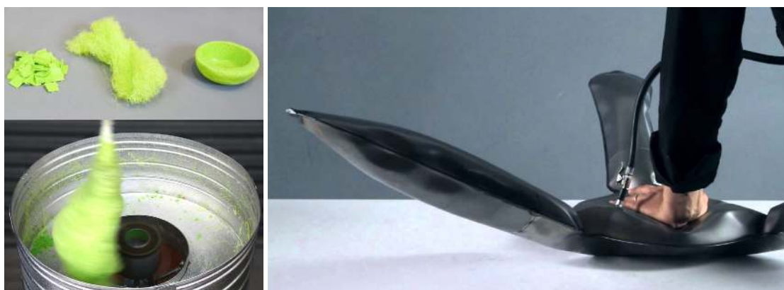
Figure 10. Repurposing and inventing tools and techniques may unlock novel material affordances: top left, fiberized and molded polypropylene waste; bottom left, Polyfloss Machine by A. Gaulard, N. Paget, C. Machet and E. De Visscher, Royal College of Art, London, 2012 (image source: The Polyfloss Factory Ltd.; reprinted with permission); right, metal inflating by Oskar Zieta, 2011 (image source: Zieta Prozessdesign; reprinted with permission).
