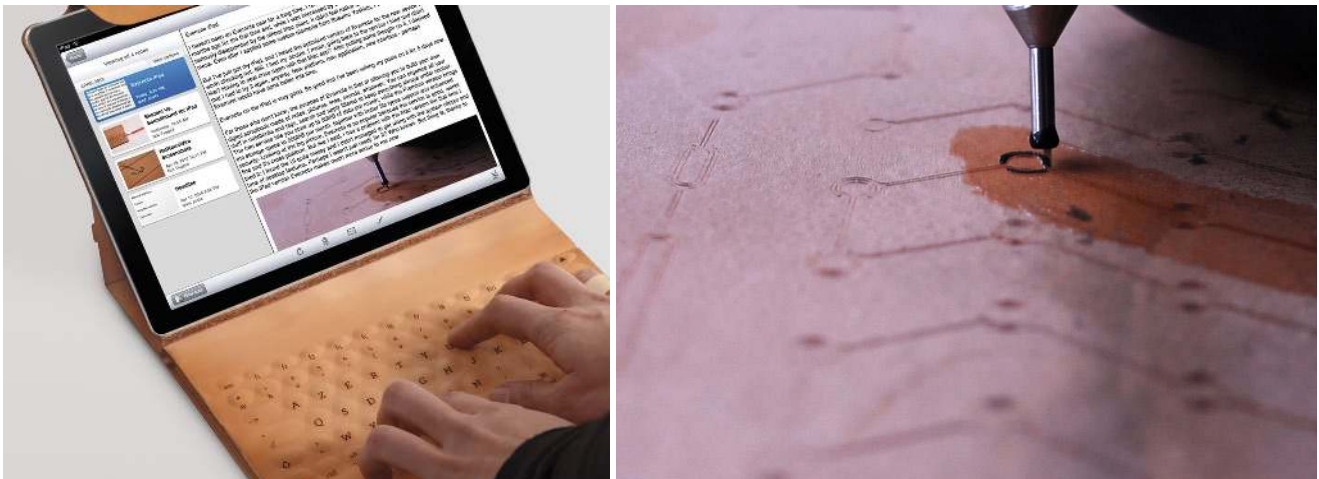
Figure 7. A novel potential of leather is unlocked through the skillful act of tattooing with conductive ink: left, iPad cover and keyboard INKO; right, the leather being tattooed with conductive ink (design and photo by Alexandre Echasseriau; tattooing by Tatoué and Jeremy Lorenzato; conductive ink: Bare Conductive; reprinted with permission).
