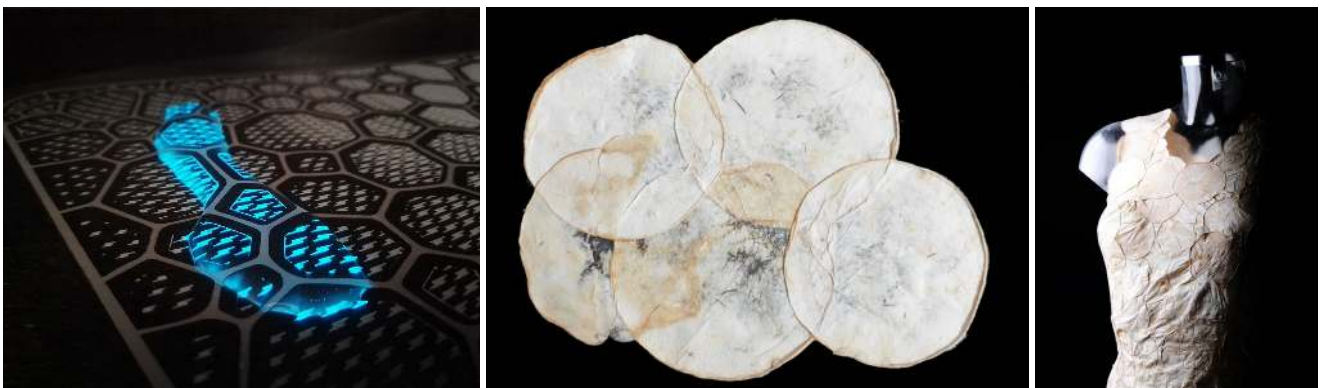
Figure 9. Discovery and perception of new affordances through materials experimentation: left, water-activated electroluminescent sample (design, fabrication, and photo by Stan Claus; reprinted with permission); right, MycoTEX textile and dress made from aggregated pure mycelium pieces by Aniela Hoitink | NEFFA (image source: Aniela Hoitink | NEFFA; reprinted with permission).
