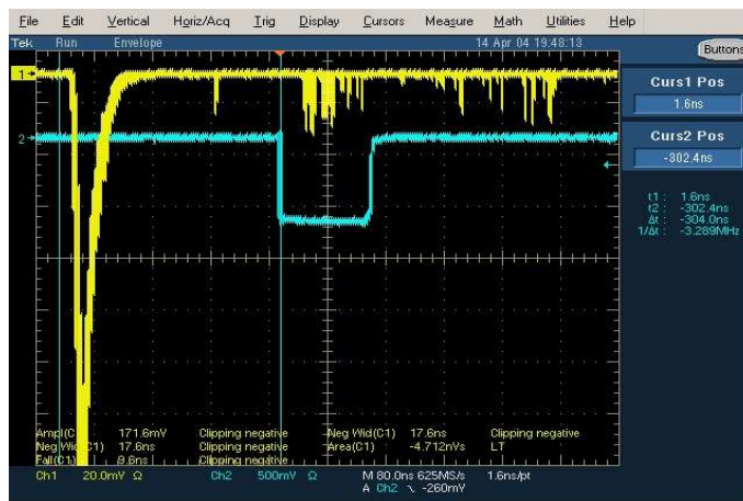
Figure 1. A sample scope view of the Hamamatsu R7525 PMT afterpulses at a gain of 10^6 . The blue line shows the 125 ns gate, the yellow line shows the signal. Both inputs are shown in envelope mode for demonstration purposes.
