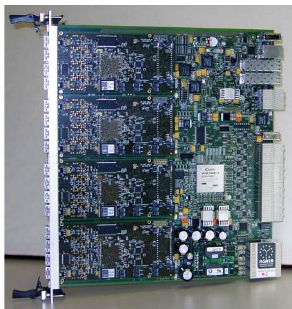
Figure 27: (Colour online) Photograph of the AGATA pre-processing ATCA carrier card.
