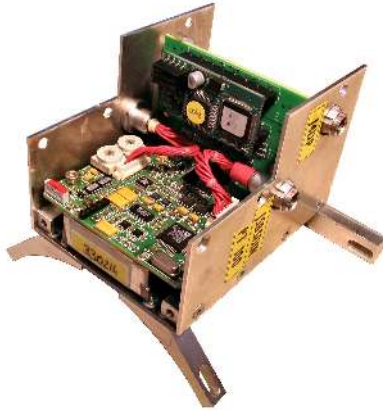
Figure 20: (Colour online) The AGATA high-voltage module composed of a compact ISEG DC/DC module and control-electronics boards including a microcontroller.
