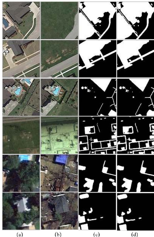
Fig. 9. CD results of AGCDetNet on the Season-Varying dataset. Zoom in for an improved view. (a) Image T1. (b) Image T2. (c) Reference change map. (d) AGCDetNet. Best viewed in color.
