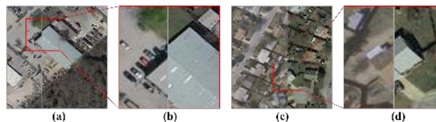
Fig. 1. Illustrations of geometric registration errors (a)–(b) and spectral changes (c)–(d). We stitched the bitemporal images together and used the red boxes to highlight the pseudo-changes. Zoom in for an improved view. (b) and (d) are the local enlarged views of (a) and (c), respectively.
