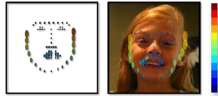
Fig. 2: Visualization of the uncertainties associated with the 68 facial feature detections. Left: Uncertainties on the reference coordinate frame. Mid: Uncertainties on a sample face image. Note that ellipses are aligned with the image axes, as we assume variance along the axes is uncorrelated. In both images color codes the amount of uncertainty; color-bar provided on the right.
