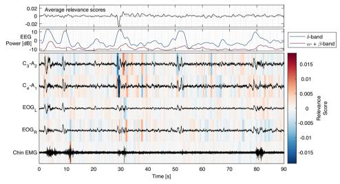
Fig. 2 Example of model (b; EEG+EOG+EMG) interpretation through relevance attribution of samples. The top plot shows relevance scores averaged across channels (C3-A2, C3-A1, EOGL, EOGR, Chin EMG). The second plot shows EEG power in the δ-band (0–4 Hz) and the combined  $\alpha$ - and  $\beta$ -bands (>8 Hz). Red and blue indicate positive and negative attribution to the age estimate, respectively. Relevance attribution was computed using gradient SHAP.
