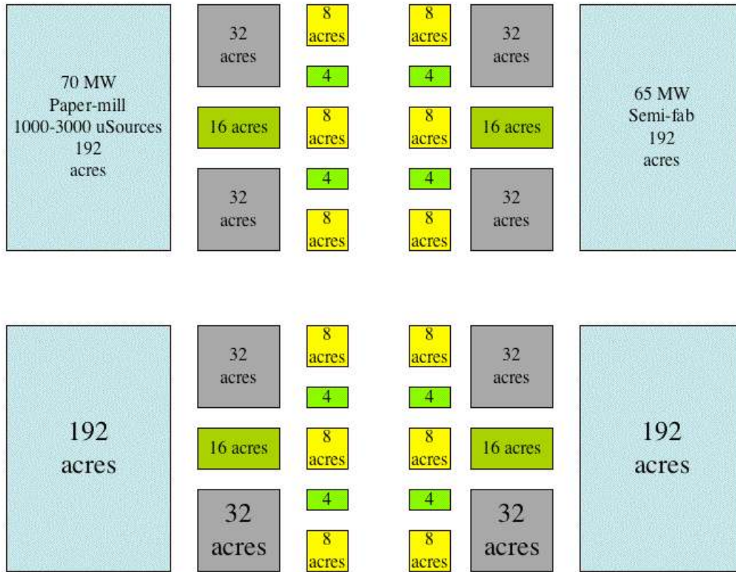
Figure 2: Notional Industrial Park Microgrid Layout
