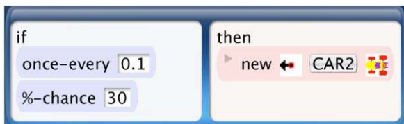
Fig. 15. Faulty behavior for the Car Generator agent. New car creation gets called too often and with high probability. There is no check for an empty spot to create the car either.
