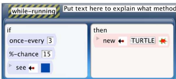
Fig. 20. Faulty turtle generation behavior. Generation frequency and chance are too low for the game to be winnable, as there are not enough turtles for the frog to jump onto to cross the river.
