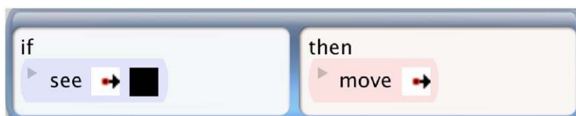
Fig. 13. Missing rule for the car to be added to the behavior in Fig. 12 to make it move right, but only if there is road ahead of it.
