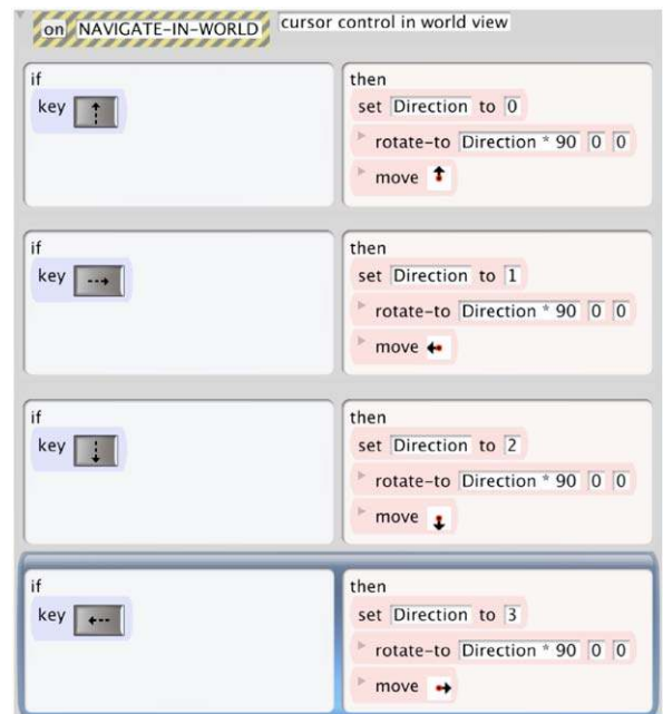
Fig. 17. Faulty behavior of 2D navigation bug. When the right and left arrow keys are pressed the frog does not move in correct direction. Notice in 2nd and 4th rule the opposite arrows checked in the key condition and the arrows of movement in the move action.
